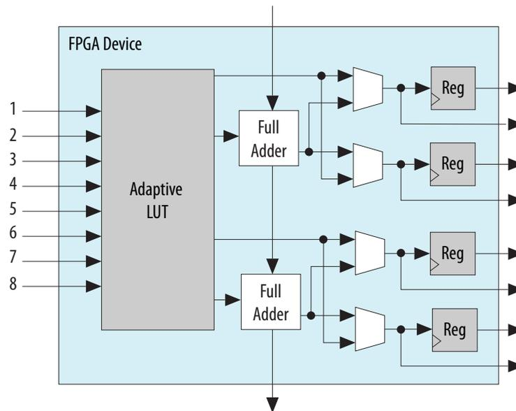
You can configure up to 50% of the ALMs in the Arria V devices as distributed memory using MLABs.
