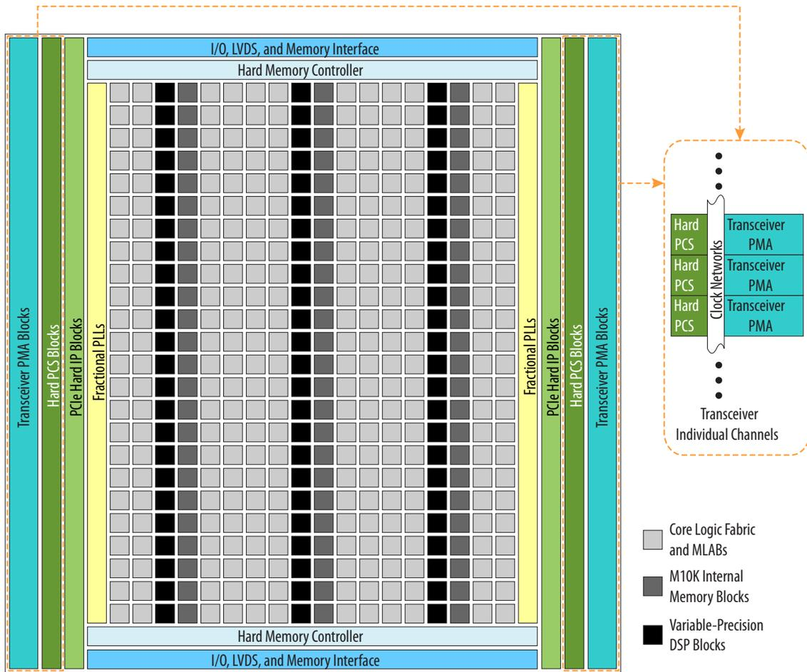
Figure 10: Device Chip Overview for Arria V GZ Devices
