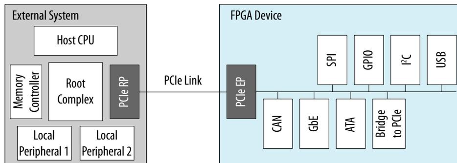
The Arria V PCIe hard IP operates independently from the core logic. This independent operation allows the PCIe link to wake up and complete link training in less than 100 ms while the Arria V device completes loading the programming file for the rest of the device.
