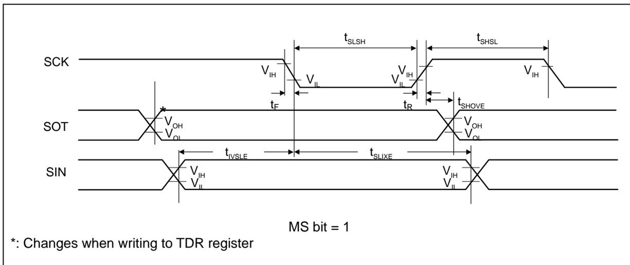
**High-Speed Synchronous Serial (SPI = 1, SCINV = 1)**
