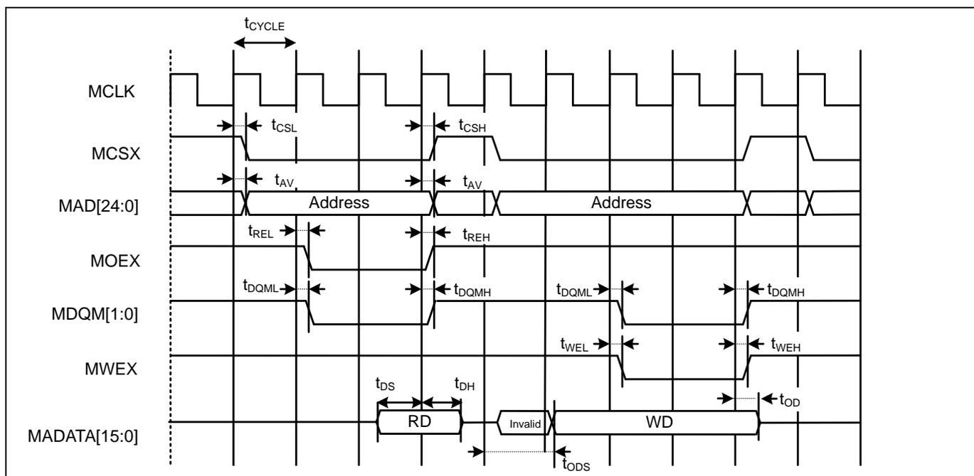
**Multiplexed Bus Access Asynchronous SRAM Mode**
