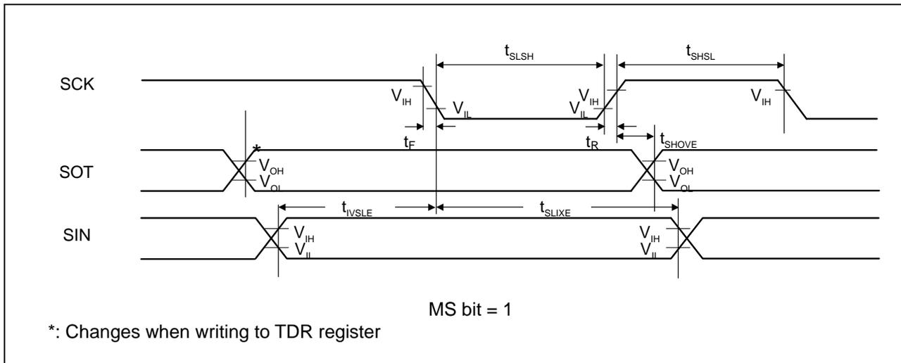
**Synchronous Serial (SPI = 1, SCINV = 1)**
