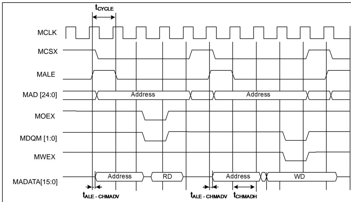
**Multiplexed Bus Access Synchronous SRAM Mode**
