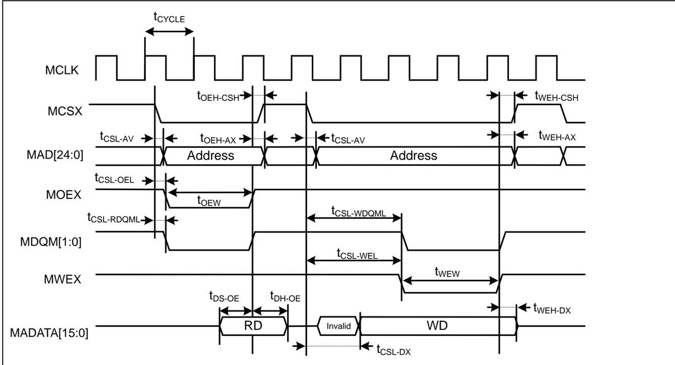
**Separate Bus Access Synchronous SRAM Mode**
