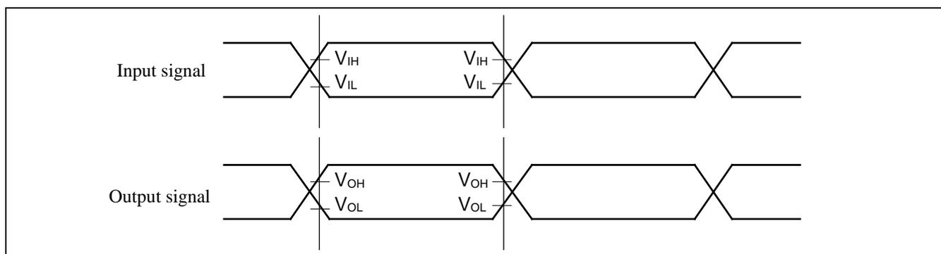
**Separate Bus Access Asynchronous SRAM Mode**
