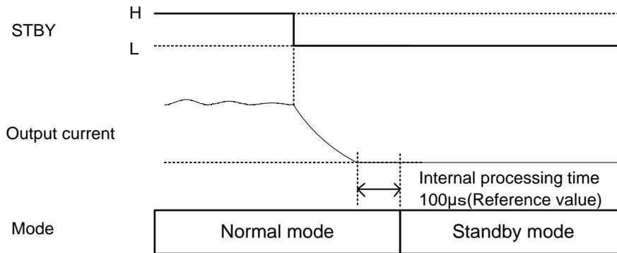
If the output current is zero-detected, the operation mode enters into the standby mode after 100 µs. The mode enters into the standby mode forcedly after 1 ms(max) from STBY=L.
