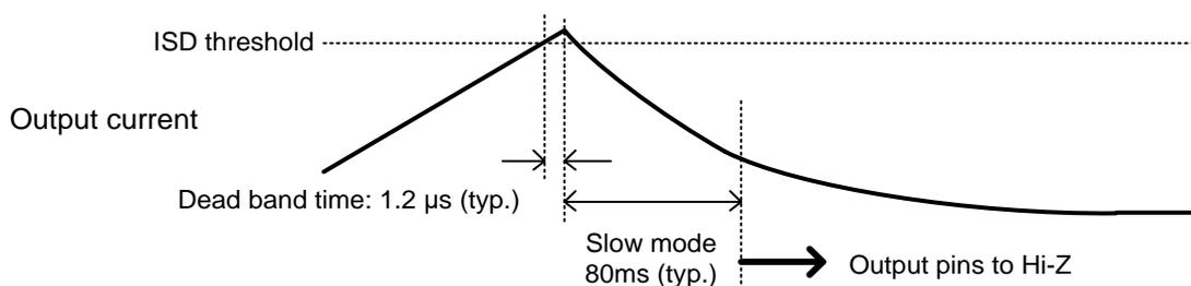
Note: Above ISD operation threshold value and band times are reference values, and are not guaranteed.
