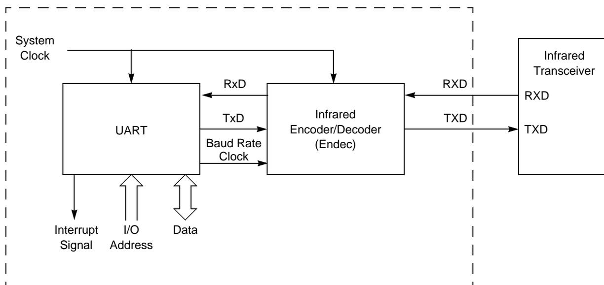
Figure 16. Infrared Data Communication System Block Diagram
