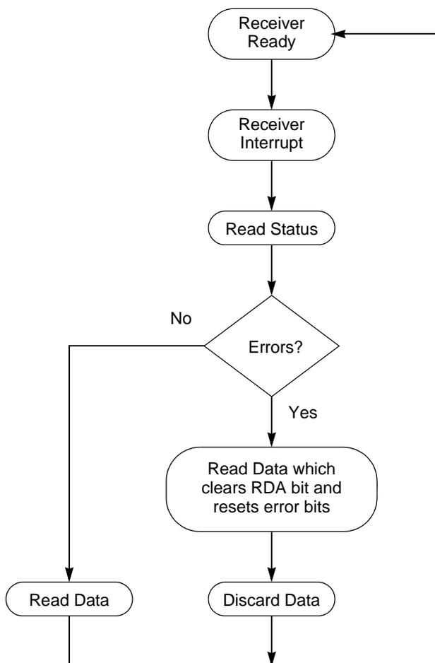
Figure 15. UART Receiver Interrupt Service Routine Flow
