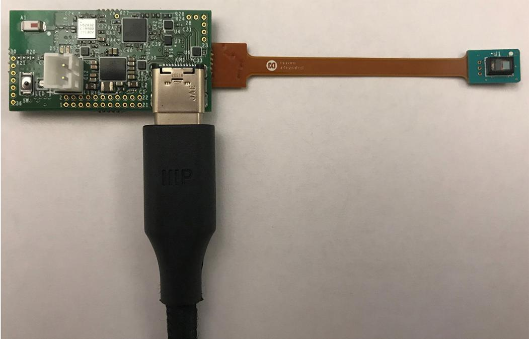
Figure 2. Hardware Setup (MAXM86161 EV System Micro PCB)
