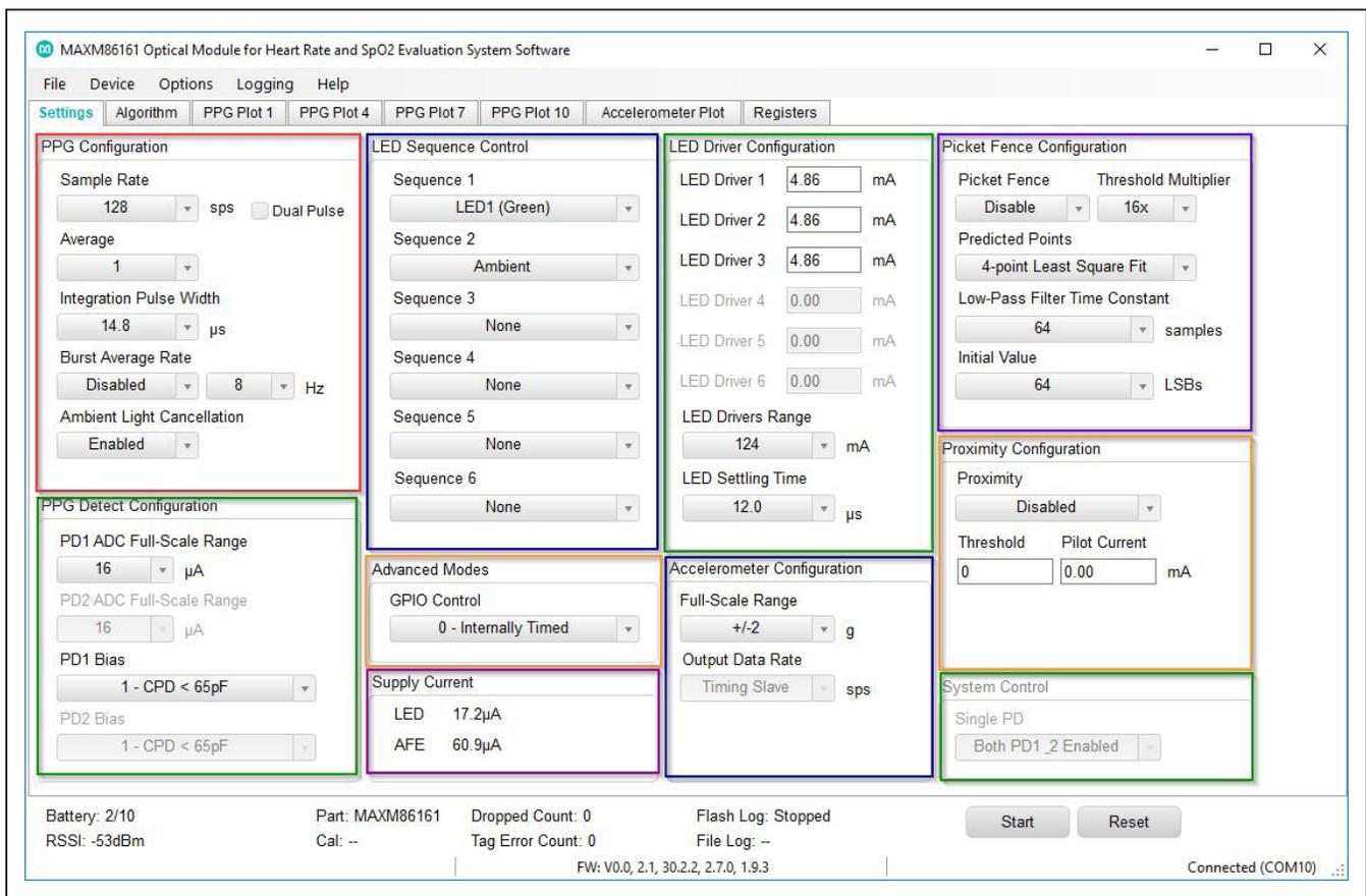
Figure 15. MAXM86161 EV System GUI: Settings Tab Descriptions
