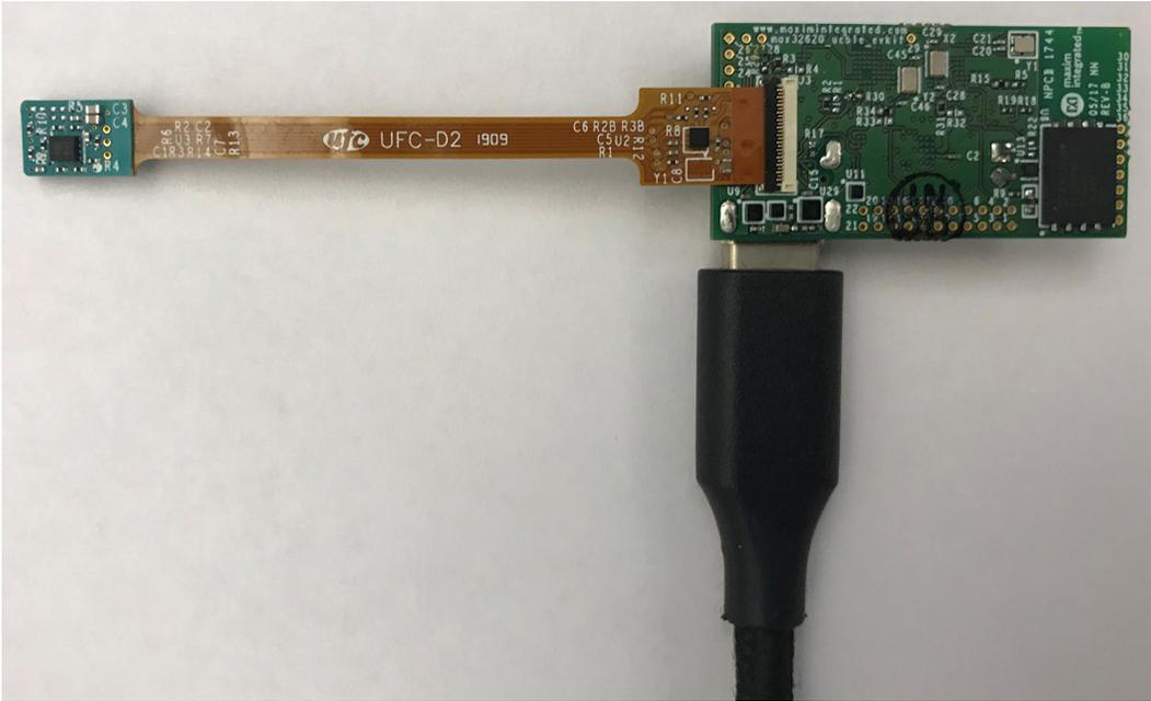
Figure 3. Hardware Setup (MAXM86161 EV System Sensor PCB)
