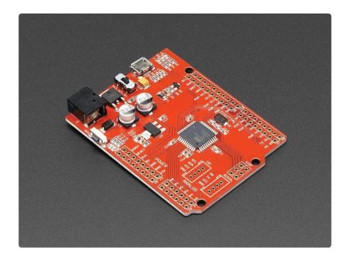
There is one little problem though. The Zumo chassis has a couple of unfortunately placed capacitors that interfere with the DC jack and capacitors on the Seeeduino. The good news is that the Seeeduino ships without headers installed. So all you need to do is replace them with slightly longer headers. The <a href="Arduino R3 Stacking">Arduino R3 Stacking</a> Headers (http://adafru.it/85) are just the thing we need.
