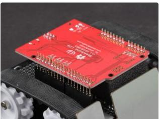
Place the Seeeduino Lite board face down over the extended headers and let it rest on the foam. There will be about 1/4" (6mm) of the header pin showing below the board.
