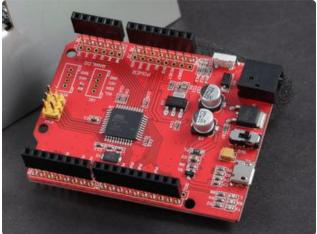
Install the 6-pin ICSP header from the Seeeduino kit from the top side and solder in place.
