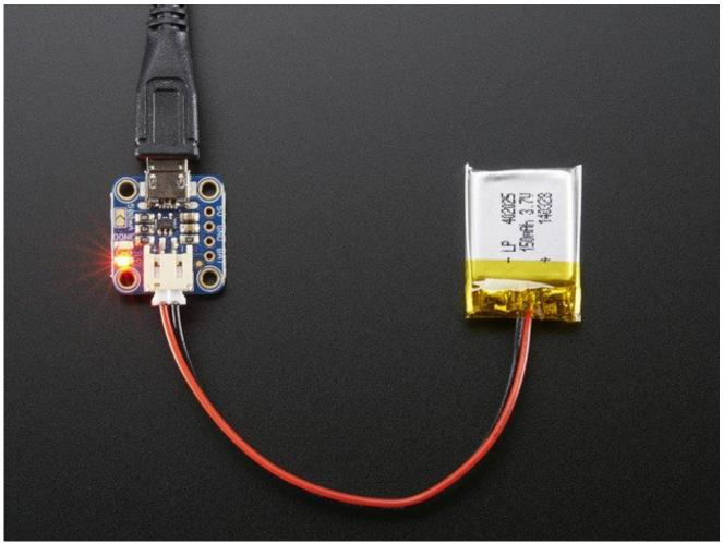
You can plug in either the battery first or the USB port first. We provide a JST jack since the large number of batteries we carry come with a JST PH connector or cable If you are soldering on a JST cable or using a non-Adafruit battery check the polarity of the wires going into the battery port. A backwards battery can destroy the charger!
