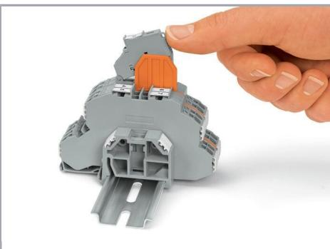
An end plate for fuse disconnect terminal blocks (shown in orange, 2002-1092) is used for additional protection, preventing the fuse holder from being opened. The fuse cannot be replaced until disconnecting the fuse holder from the power supply.
