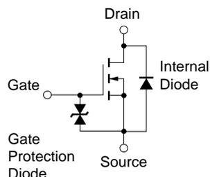
**Remark** The diode connected between the gate and source of the transistor serves as a protector against ESD. When this device is actually used, an additional protection circuit is externally required if a voltage exceeding the rated voltage may be applied to this device.
