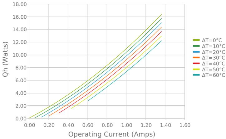
Total Heat Dissipated at Hot Side (Qh=Qc+Pin)
