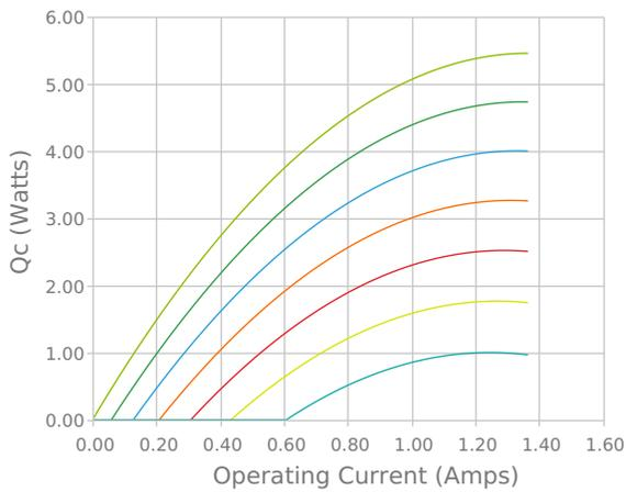
Heat Pumped at Cold Side
