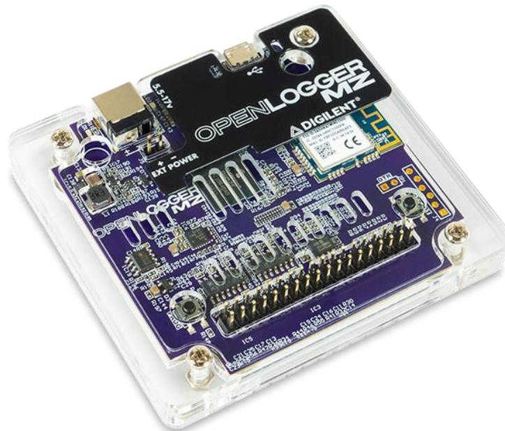
OpenLogger is a wireless data logging and data acquisition device that can be controlled via USB or WiFi. Using a computer or mobile device, signals from circuits and sensors can be acquired, stored, analyzed, visualized, and generated. OpenLogger makes it easy to monitor multiple analog inputs and simultaneously log the data to an SD card, and/or stream over USB or WiFi, all through [WaveForms Live](#).
