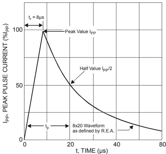
Figure 1 Pulse Waveform
