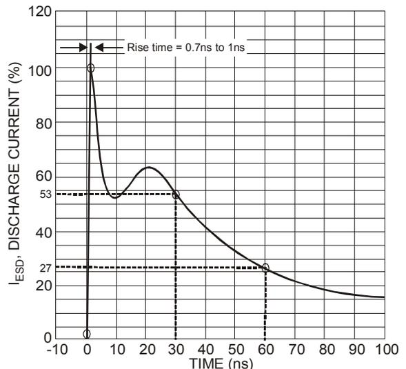
Figure 2 ESD Discharge Current Wave Form
