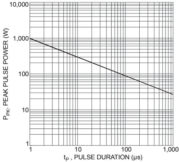
Figure 3 Peak Pulse Power vs. Pulse Duration
