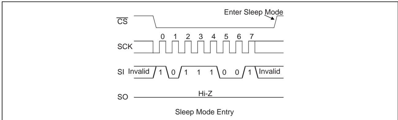
Returning to a normal operation from the SLEEP mode is carried out after  $t_{REC}$  (Max 400  $\mu$ s) time from the falling edge of  $\overline{CS}$  (see the figure below). It is possible to return  $\overline{CS}$  to H level before  $t_{REC}$  time. However, it is prohibited to bring down  $\overline{CS}$  to L level again during  $t_{REC}$  period.
