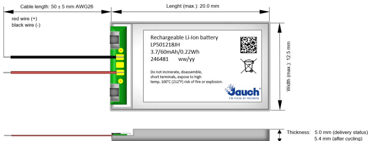
Important Note: Due to the small size and low capacity of this battery, please charge the battery before use, to avoid deep discharge. If the battery shows 0V, the overvoltage protection has kicked in. To wake the battery, complete a full charge cycle.
