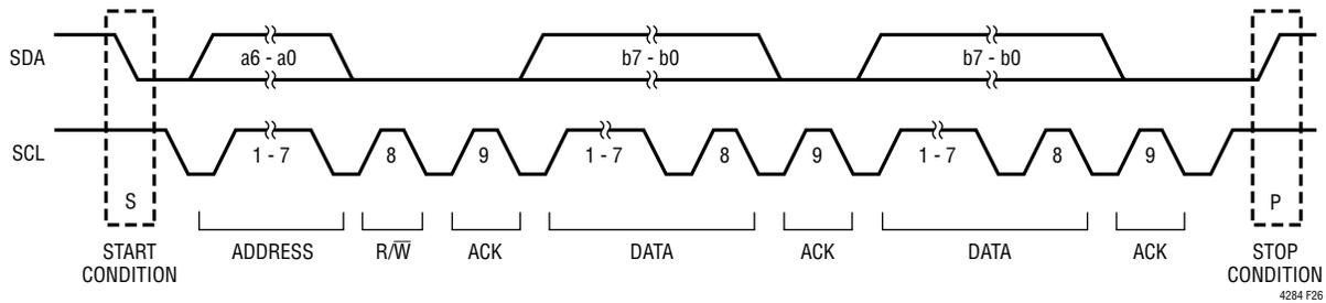
Figure 26. General Data Transfer over I<sup>2</sup>C
