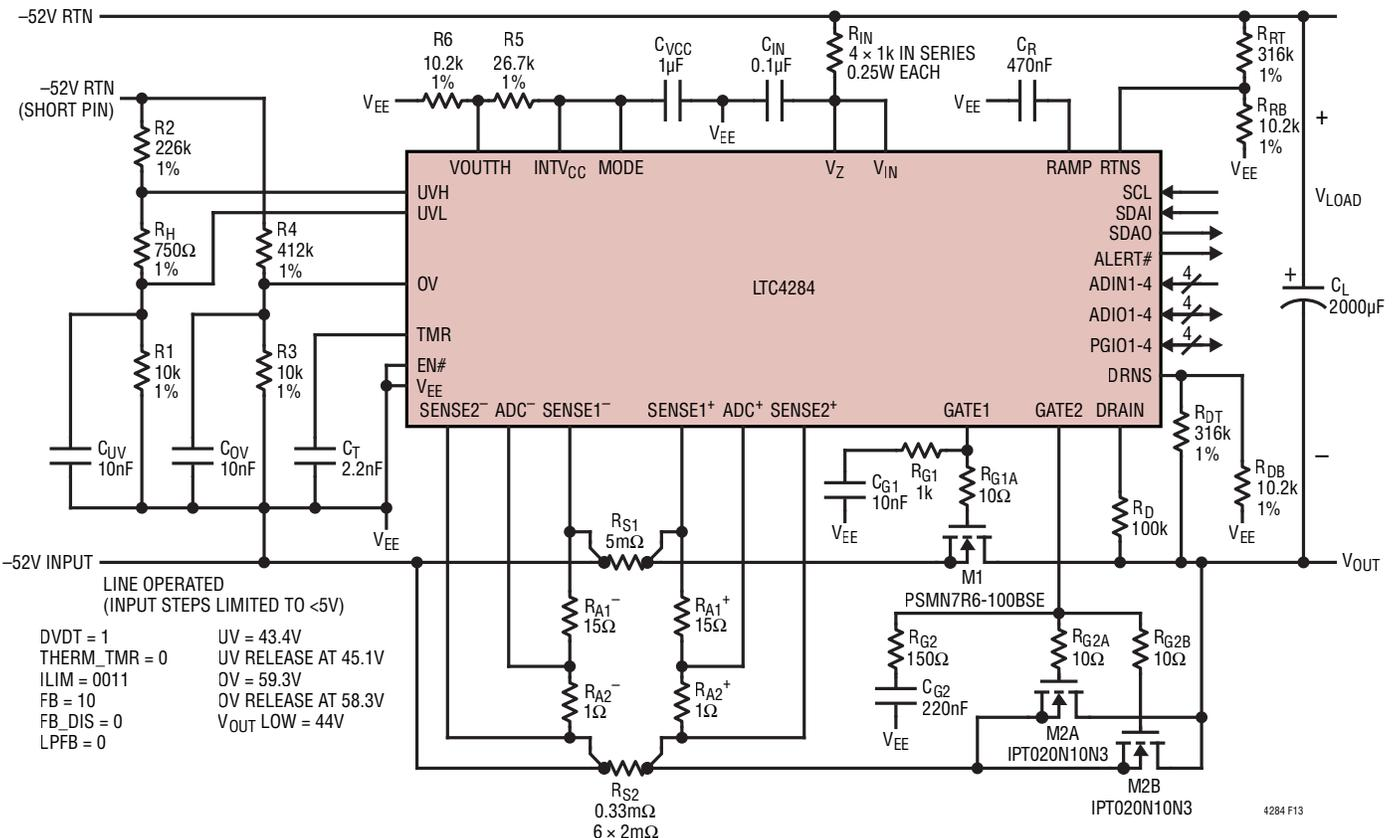
**Figure 13. -52V/2500W Hot Swap Controller in Low Stress Staged Start Mode with dV/dt Inrush Control: GATE1 Drives Trickle Startup MOSFET and GATE2 Drives Low  $R_{DS(ON)}$  MOSFETs, for Systems with Tightly Regulated Supply Voltages**
