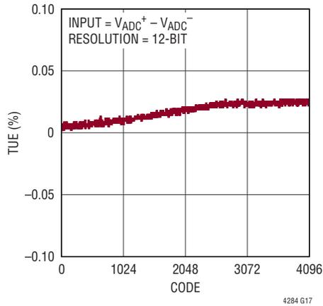
**12-Bit Voltage ADC INL vs Code**
