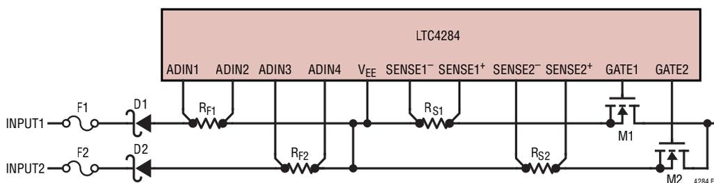
Figure 24. Individual Feed Current and Channel Current Monitoring
