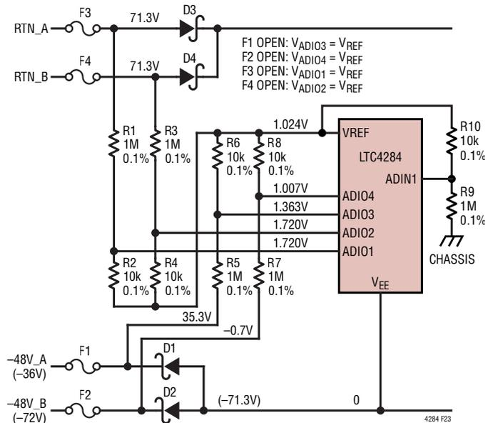
Figure 23. Feed Voltage and Open Fuse Monitoring
