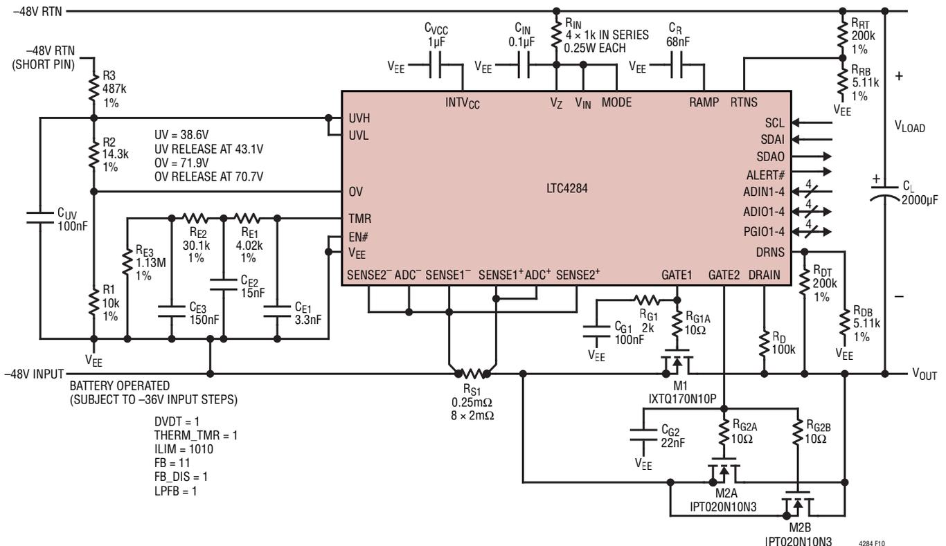
**Figure 10. -48V/1800W Hot Swap Controller with SOA Timer and dV/dt Inrush Control in High Stress Staged Start Mode: GATE1 Drives High SOA MOSFET and GATE2 Drives Low R<sub>DS(ON)</sub> MOSFETs**
