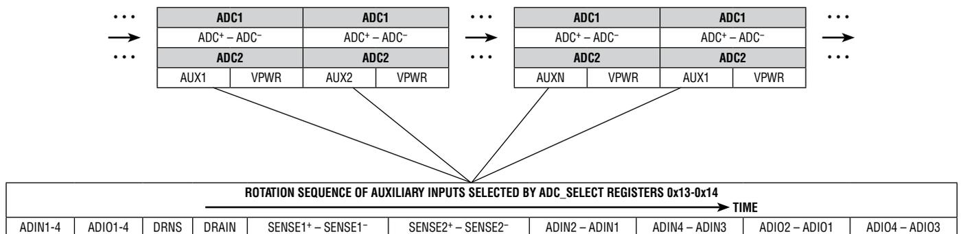
Figure 21. LTC4284 ADC Measurement Pattern in Continuous Mode
