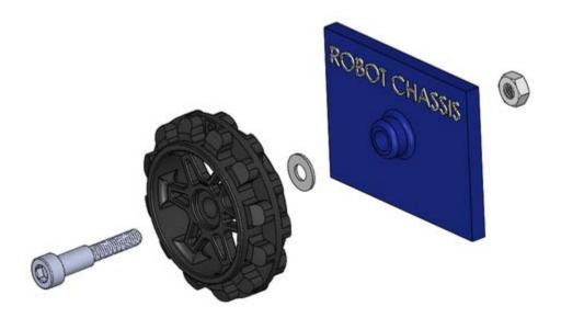
Included are two pairs of shoulder bolts, one with a 5mm threaded portion and one a 12mm threaded portion, so you can pick the pair that is appropriate for your application. You will only use two of the four included shoulder bolts.
