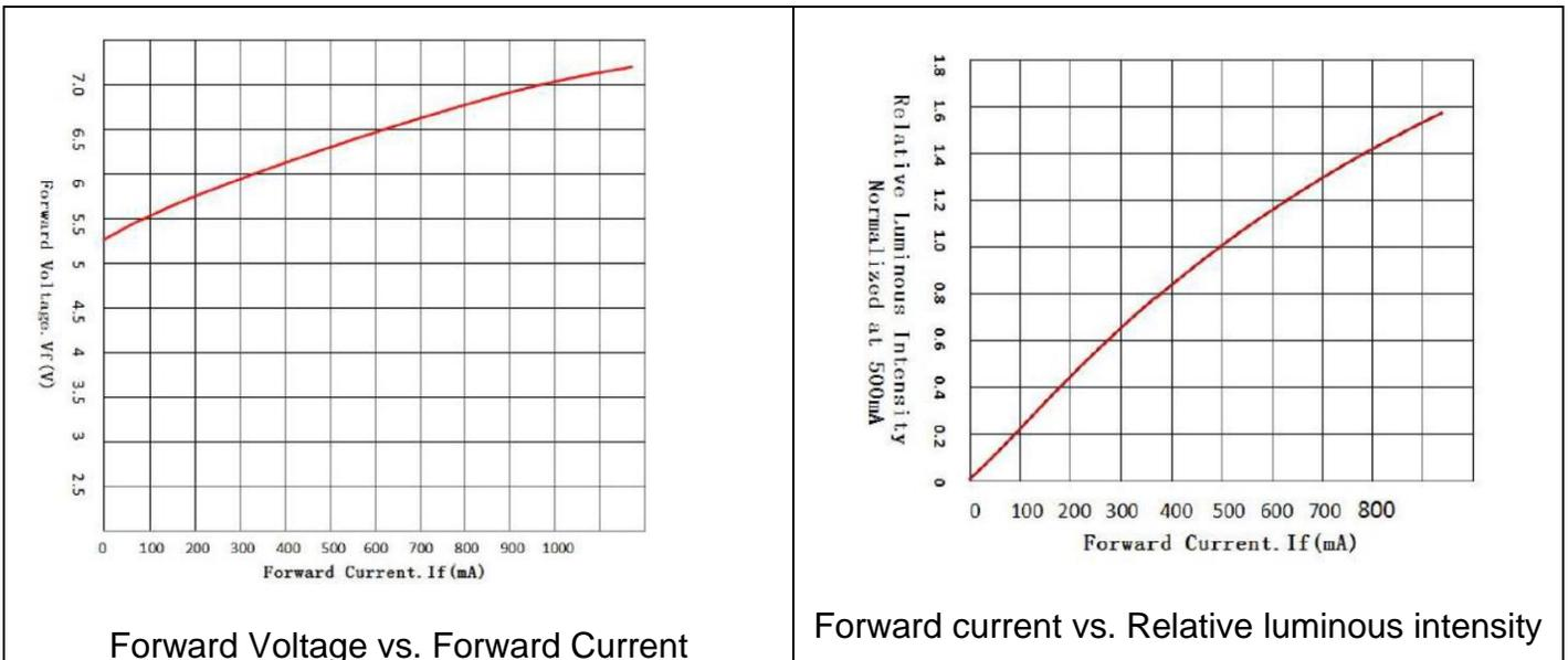
Forward Voltage vs. Forward Current
