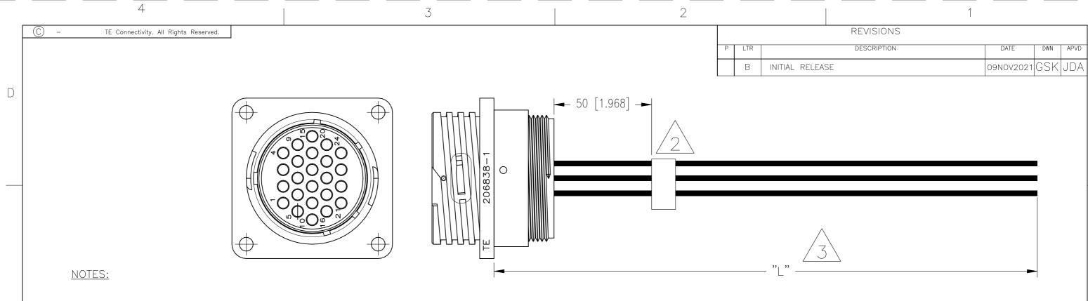
1. OVERALL INSULATION CRIMP DIAMETER, INCLUDING CRIMP BARREL, MUST NOT EXCEED .125 [3.18]
