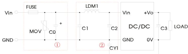
Notes: We use Part „1“ in Fig. 3 for immunity and part „2“ for emissions test. Selecting based on needs.
