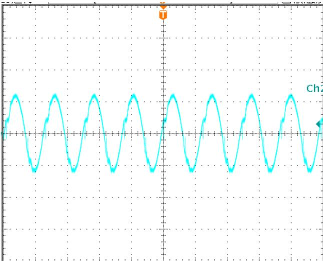
**Figure 14:** Output voltage ripple at nominal input voltage and max load current (20 mV/div, 2 µs/div)
