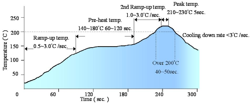
Note: The temperature refers to the pin of V48SC, measured on the pin +Vout joint.
