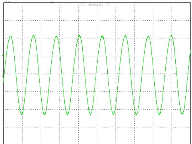
**Figure 11:** Input Terminal Ripple Current,  $i_c$ , at max output current and nominal input voltage with  $12\mu H$  source impedance and  $33\mu F$  electrolytic capacitor ( $100mA/div$ ,  $2\mu s/div$ ).
