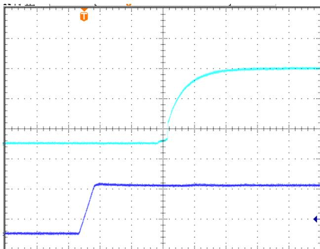
**Figure 6:** Turn-on transient at zero load current (10 ms/div).
