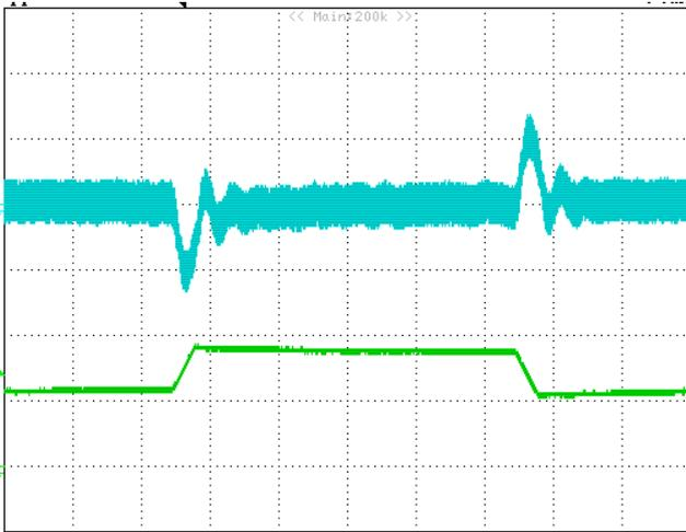
**Figure 8:** Output voltage response to step-change in load current (50%-75%-50% of full load;  $di/dt = 0.1A/\mu s$ ). Load cap:  $10\mu F$ , tantalum capacitor and  $1\mu F$  ceramic capacitor. Top Trace:  $V_{out}$ ;  $100mV/div$ ; Bottom Trace: output current:  $5A/div$ , Time:  $100\mu s/div$
