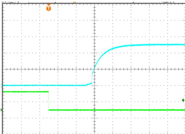
**Figure 4:** Turn-on transient at zero load current (10ms/div).
