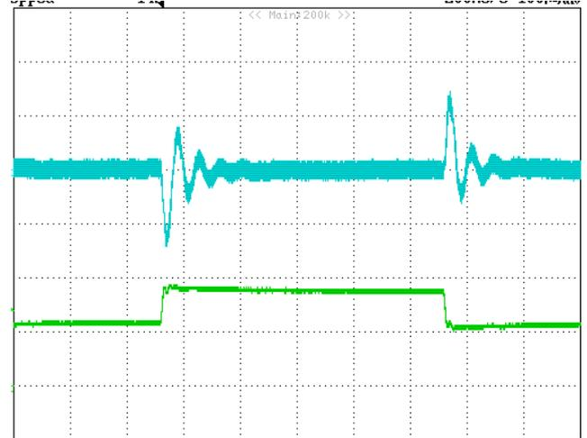
**Figure 9:** Output voltage response to step-change in load current (50%-75%-50% of full load;  $di/dt = 2.5A/\mu s$ ). Load cap:  $10\mu F$ , tantalum capacitor and  $1\mu F$  ceramic capacitor. Top Trace:  $V_{out}$ ;  $200mV/div$ ; Bottom Trace: output current:  $5A/div$ , Time:  $100\mu s/div$
