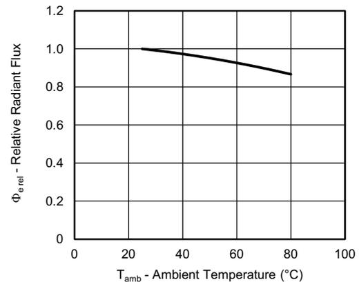
Fig. 6 - Relative Radiant Flux vs. Ambient Temperature
