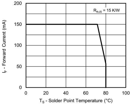
Fig. 1 - Maximum Forward Current vs. Solder Point Temperature
