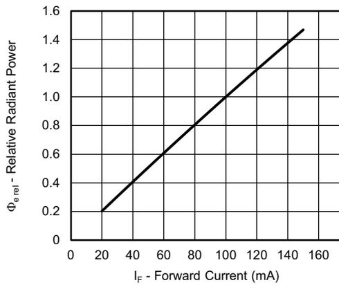
Fig. 2 - Relative Radiant Power vs. Forward Current
