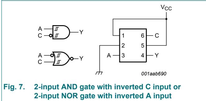
Fig. 7. 2-input AND gate with inverted C input or 2-input NOR gate with inverted A input
