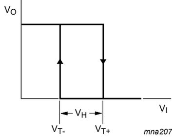
Fig. 14. Transfer characteristics
