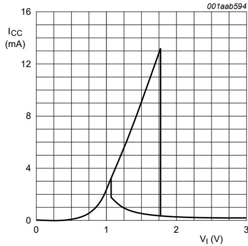
Fig. 18. Typical 74LVC1G58 transfer characteristics;  $V_{CC} = 3.0$  V
