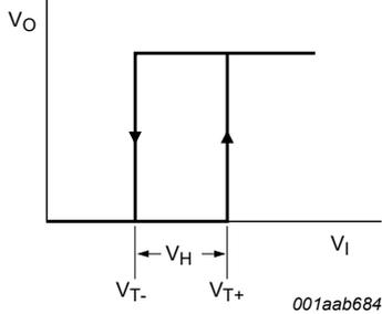
Fig. 16. Transfer characteristics
