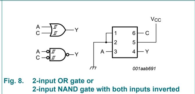
Fig. 8. 2-input OR gate or 2-input NAND gate with both inputs inverted
