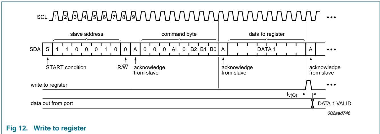
Fig 12. Write to register
