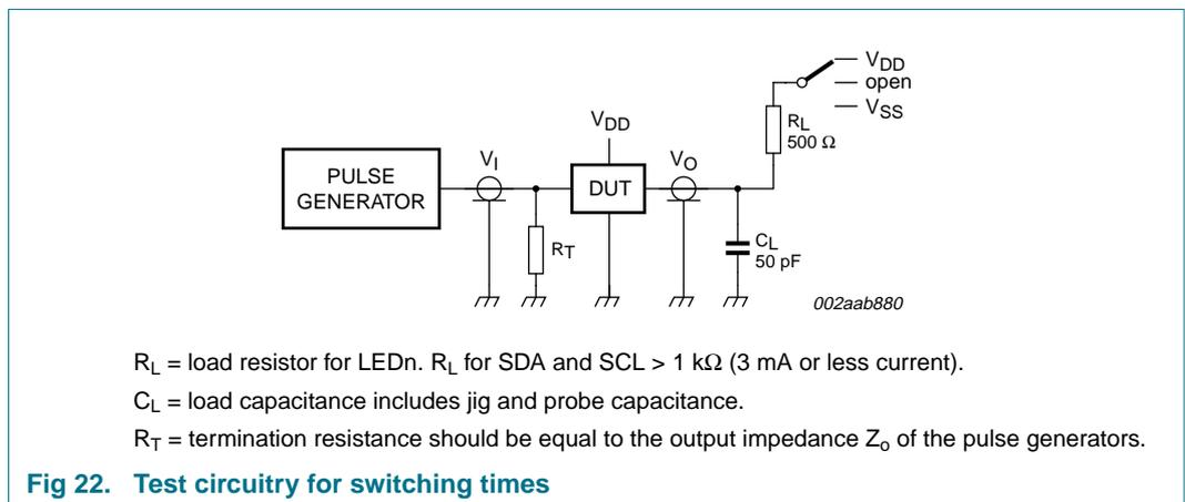
$R_L$  = load resistor for LEDn.  $R_L$  for SDA and SCL > 1 k $\Omega$  (3 mA or less current).
