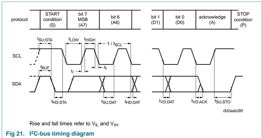
Fig 21. I<sup>2</sup>C-bus timing diagram
