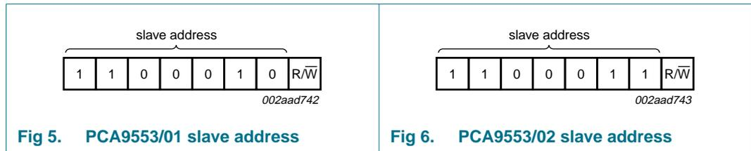
The last bit of the address byte defines the operation to be performed. When set to logic 1 a read is selected, while a logic 0 selects a write operation.
