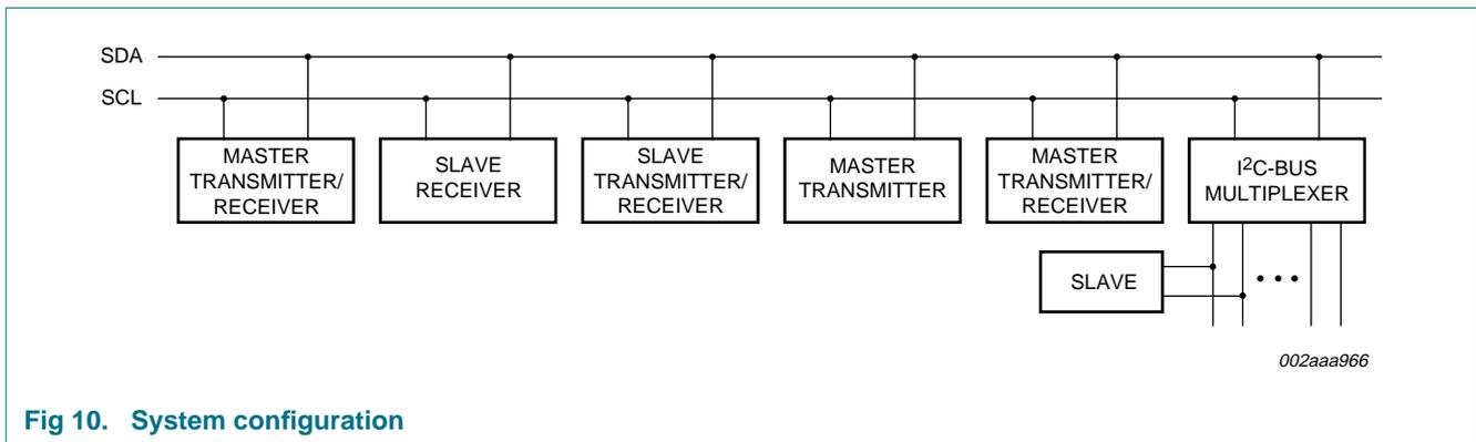
Fig 10. System configuration
