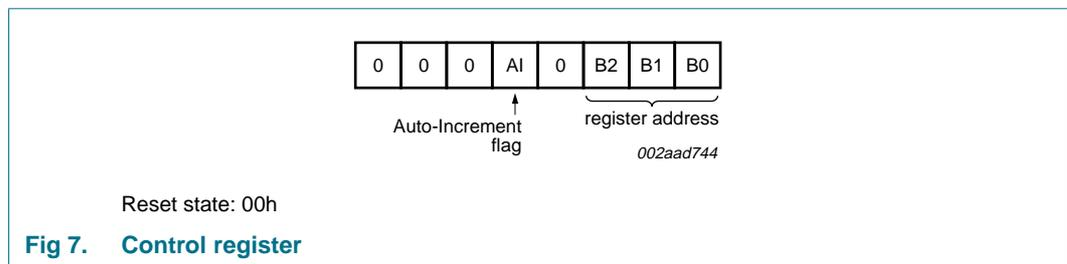
The lowest 3 bits are used as a pointer to determine which register will be accessed.
