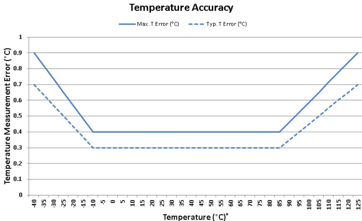
**Figure 3. Temperature Accuracy\***
