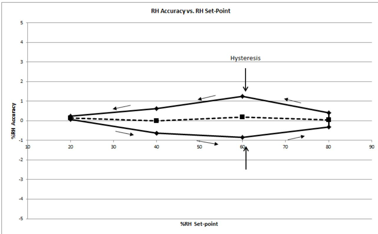
**Figure 9. Measuring Sensor Accuracy Including Hysteresis**
