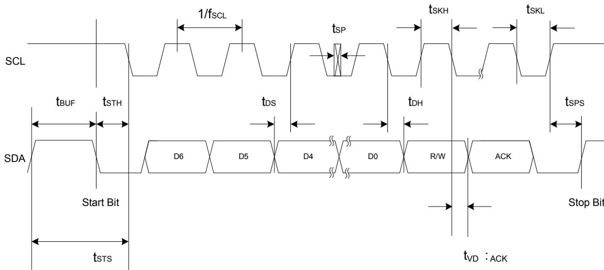
**Figure 1. I<sup>2</sup>C Interface Timing Diagram**
