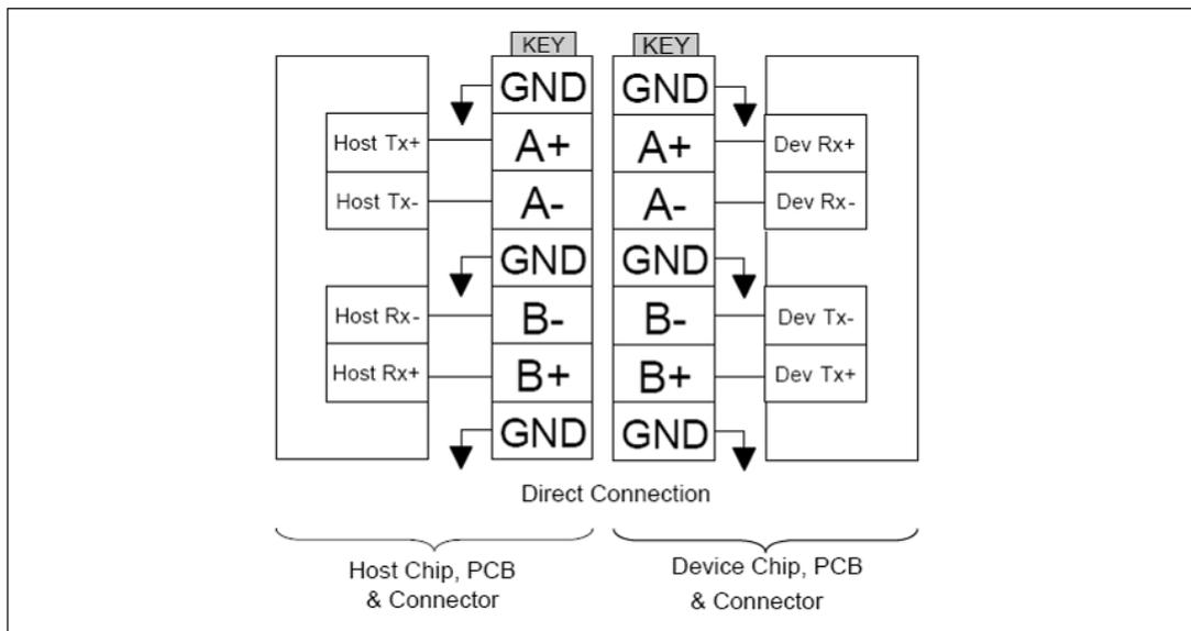
Figure 3-1 Direct Connection between the Host and Device
