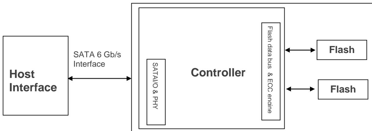
Figure 2-1 Block Diagram
