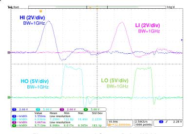
Figure 8-2. Input and Output Pulse Width
