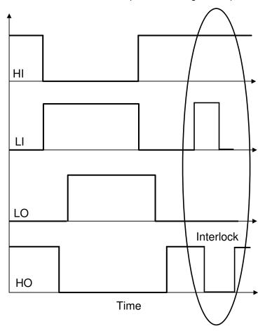
Figure 7-1. Interlock or Input Shoot-through Protection
