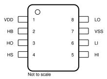
Figure 5-2. D Package 8-Pin SOIC Top View
