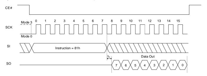
Figure 8.47 Read Extended Read Parameters QPI Sequence
