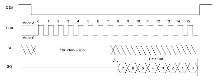
Figure 8.31 Read Function Register QPI Sequence
