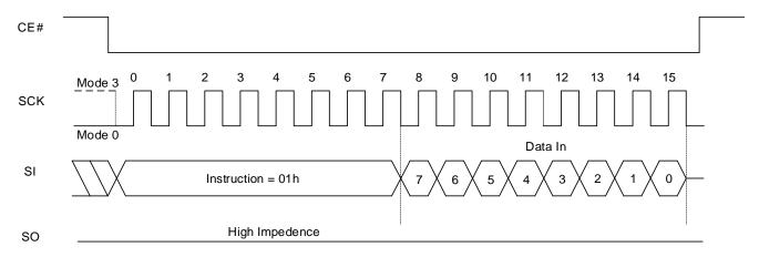
Figure 8.29 Write Status Register QPI Sequence
