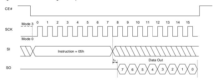
Figure 8.27 Read Status Register QPI Sequence
