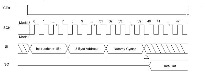
Note: Dummy cycles depends on Read Parameter setting. Detailed information in Table 6.11 Read Dummy Cycles.
