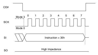
Figure 8.35 Exit Quad Peripheral Interface (QPI) Mode Sequence
