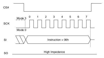
Figure 8.23 Write Enable QPI Sequence
