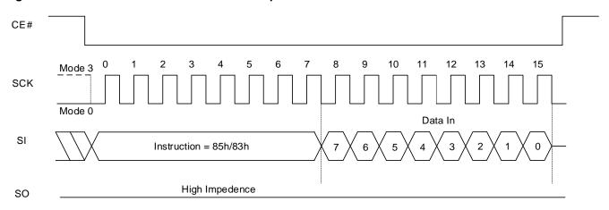
Figure 8.43 Set Extended Read Parameters QPI Sequence
