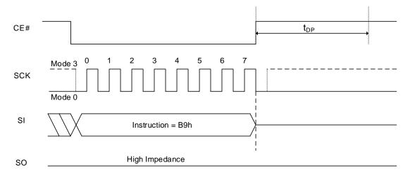
Figure 8.37 Enter Deep Power Down Mode QPI Operation
