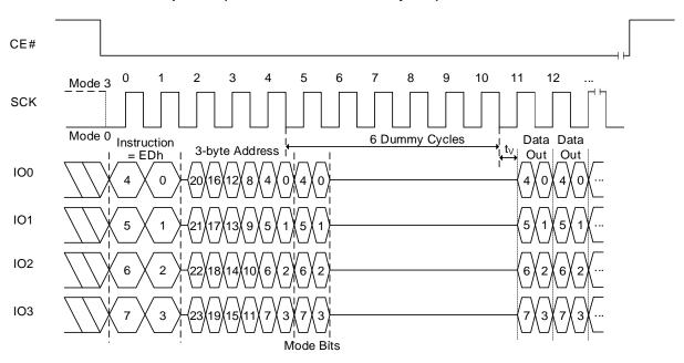
Figure 8.67 FRQDTR QPI Sequence (with command decode cycles)
