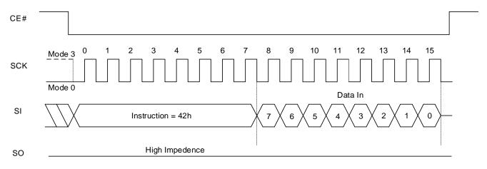
Figure 8.33 Write Function Register QPI Sequence
