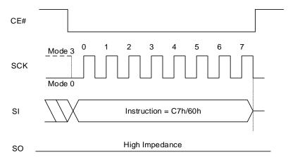
Figure 8.21 Chip Erase QPI Sequence
