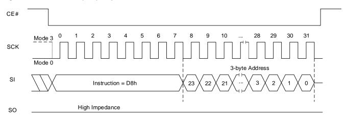
Figure 8.17 Block Erase (64K) QPI Sequence
