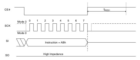
Figure 8.39 Release Deep Power Down Mode QPI Operation
