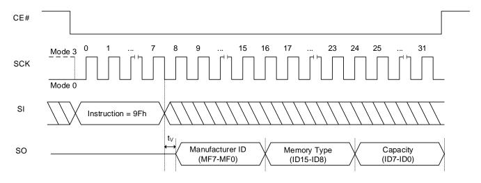
Figure 8.51 RDJDIDQ (Read JEDEC ID in QPI Mode) Sequence
