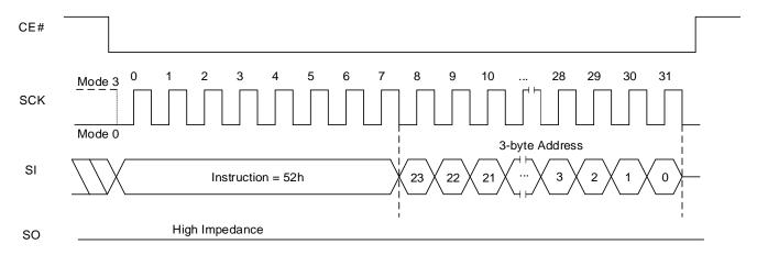
Figure 8.19 Block Erase (32K) QPI Sequence
