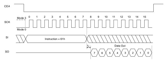
Figure 8.45 Read Read Parameters QPI Sequence
