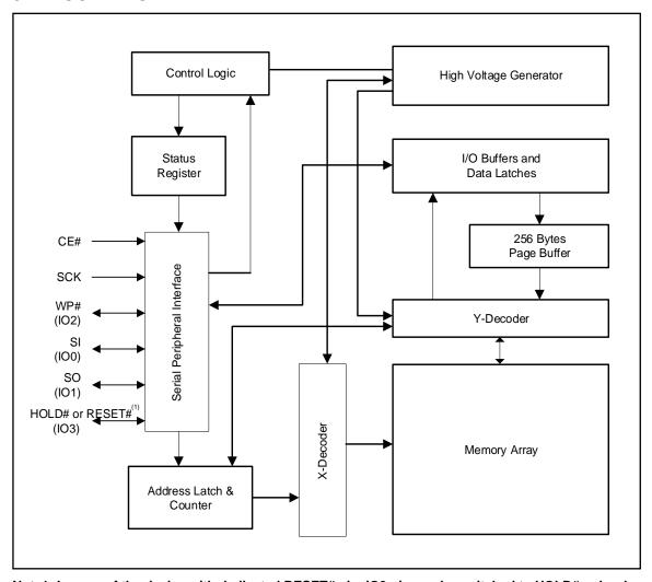
Note1: In case of the device with dedicated RESET# pin, IO3 pin can be switched to HOLD# only when QE bit=0
