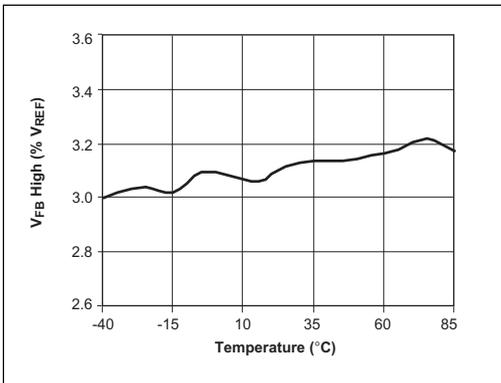
Figure 12.  $V_{FB}$  3% High Comparator vs. Temperature
