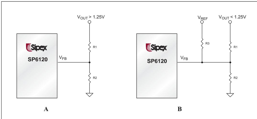
Figures 21(A), a voltage divider connected to the  $V_{FB}$  pin programs the output voltage and 21(B), a simple circuit using one external voltage reference programs the output voltages to less than 1.25V.
