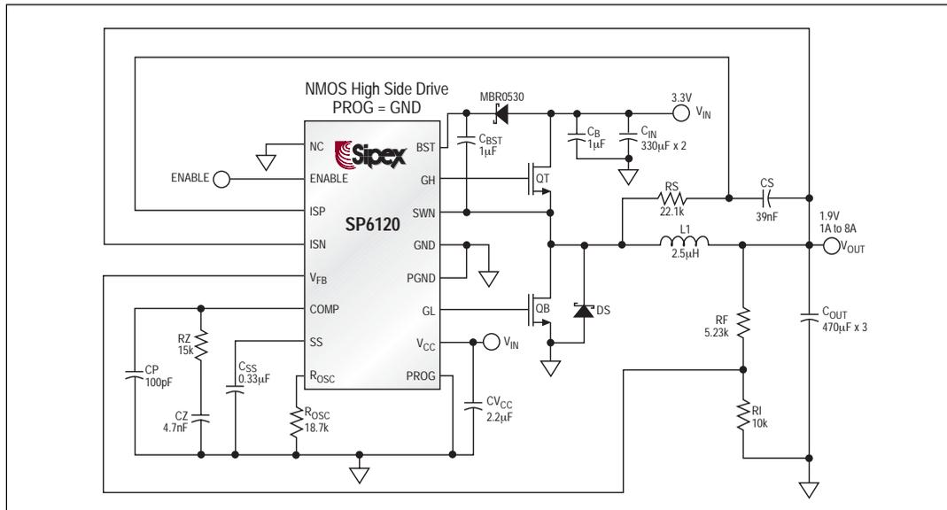
Figure 1. Schematic 3.3V to 1.9V Power Supply
