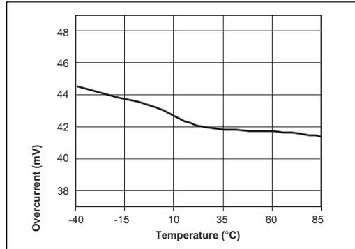
Figure 9. Overcurrent Comparator Threshold Voltage vs. Temperature
