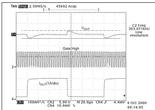
Figure 4. Load Step Response: 0.4A to 2A
