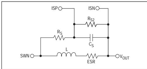
Figure 20: Current Sensing
