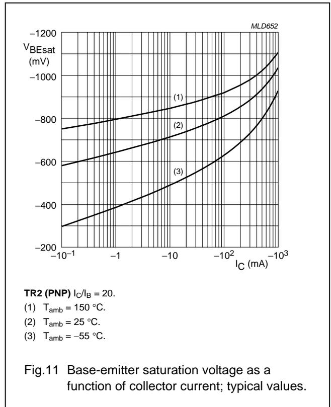
15 V low  $V_{CE(sat)}$  NPN/PNP transistor
