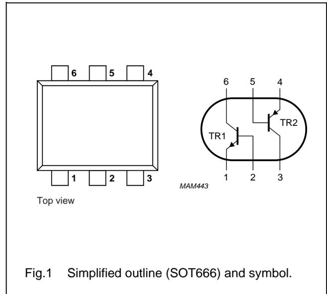
15 V low  $V_{CE(sat)}$  NPN/PNP transistor
