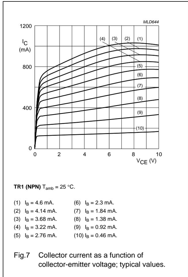
15 V low  $V_{CE(sat)}$  NPN/PNP transistor
