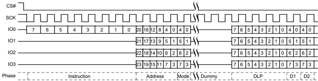
Figure 71. DDR Quad I/O Read Initial Access (4-Byte Address, EEh or EDh [CR2V[7]=1])<sup>[49]</sup>
