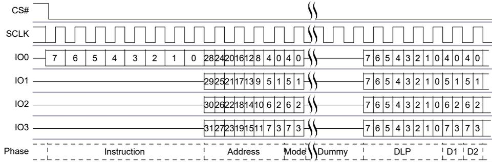
Figure 15. DDR Quad I/O Read in QPI Mode
