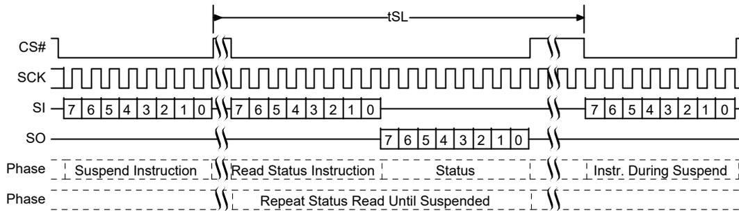
Figure 84. Erase or Program Suspend Command Sequence
