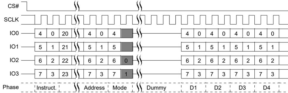
**Figure 68. Quad I/O Read Command Sequence (4-Byte Address, ECh or EBh [CR2V[7]=1])**
