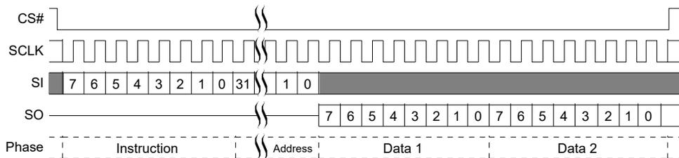
Figure 10. Single Bit Wide I/O Command with Latency
