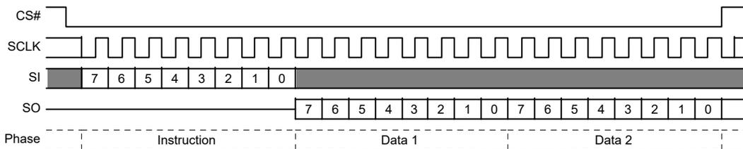
Figure 9. Single Bit Wide I/O Command without latency
