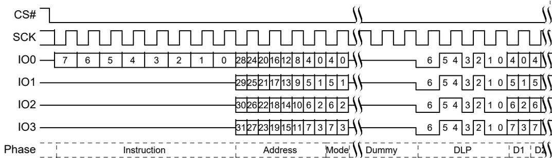
Figure 72. DDR Quad I/O Read Initial Access (4-Byte Address, EEh or EDh [CR2V[7]=1]) QPI Mode<sup>[50]</sup>
