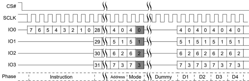
Figure 13. Quad I/O Read Command in QPI Mode
