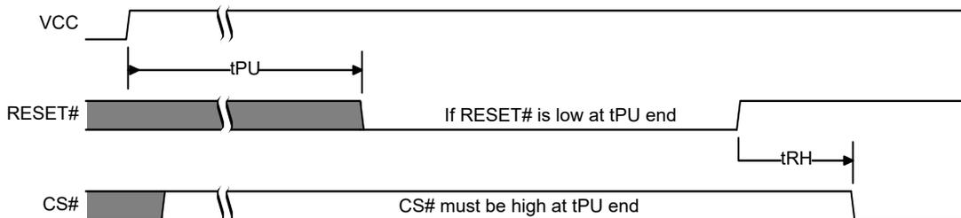
Figure 24. Reset HIGH at the end of POR
