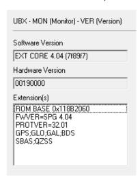
Figure 4: Checking XPLR-M9 firmware version from u-center
