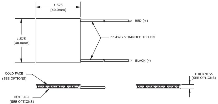
Ceramic Material: Alumina (Al<sub>2</sub>O<sub>3</sub>)
