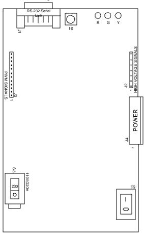
Figure 3 Connectors and indicators layout
