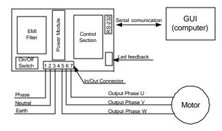
Figure 2 Typical Connection Diagram
