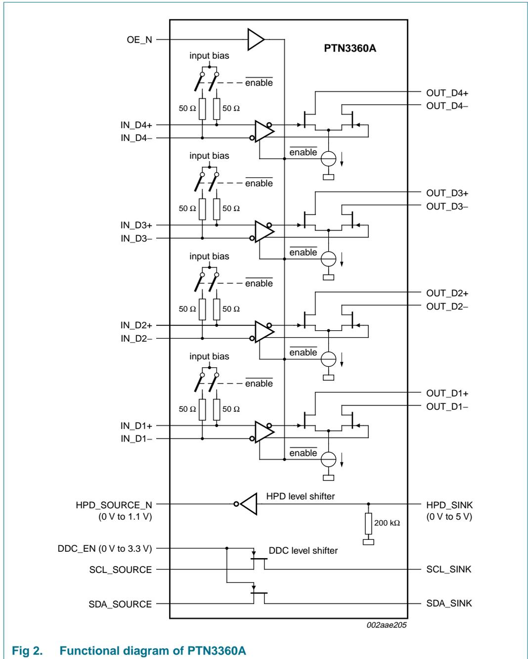
Fig 2. Functional diagram of PTN3360A
