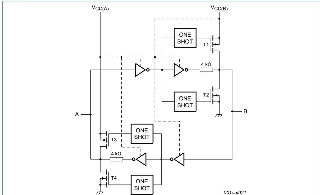
Fig. 8. Architecture of NXB0102-Q100 I/O cell (one channel)
