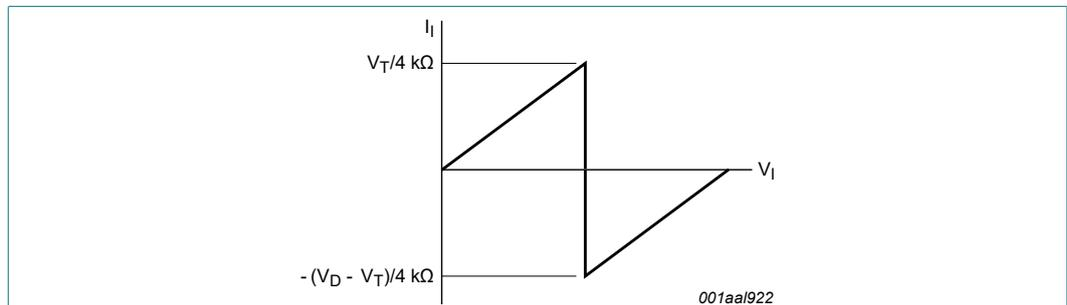
$V_T$ : input threshold voltage of the NXB0102-Q100 (typically  $V_{CCI} / 2$ ).
