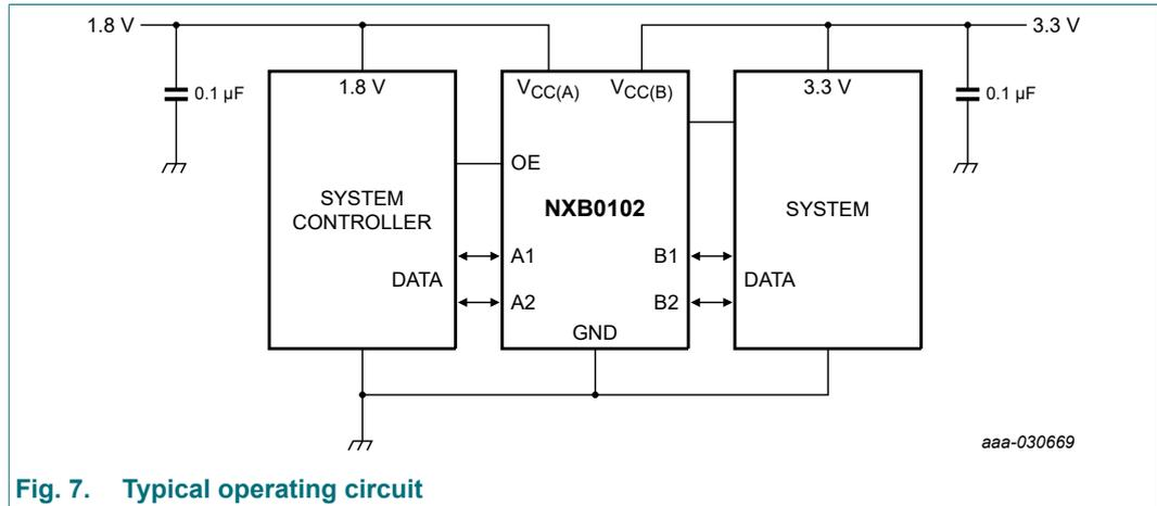
**Fig. 7.** Typical operating circuit
