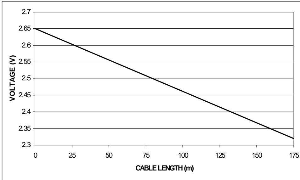
Figure 3. CLI Output Voltage Vs Belden 1694A Cable Length at SD-SDI and HD-SDI Data Rates
