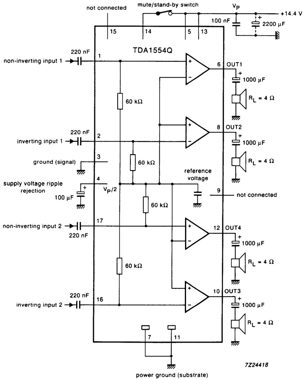
Fig.4 Quad single-ended application circuit diagram.
