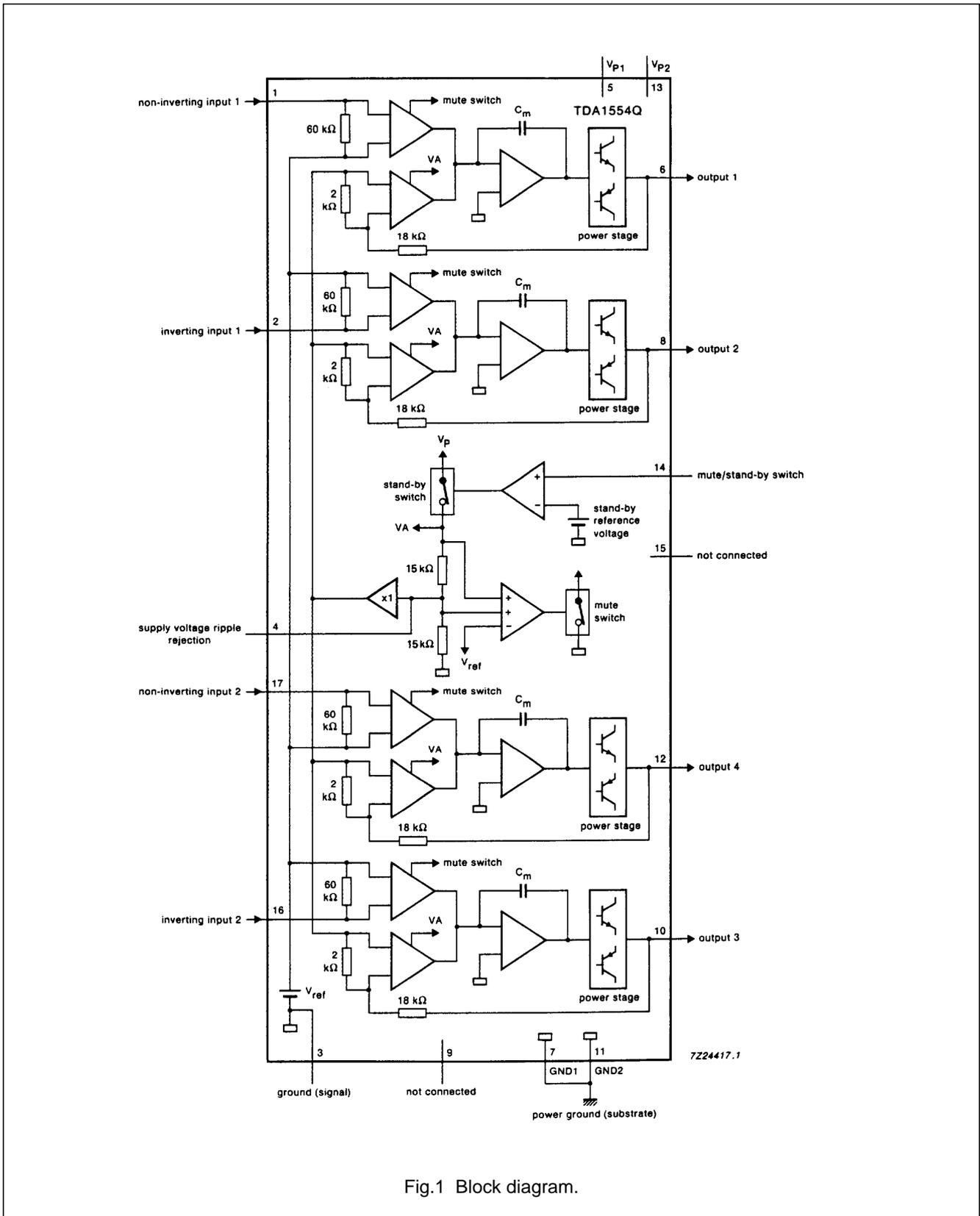
Fig.1 Block diagram.
