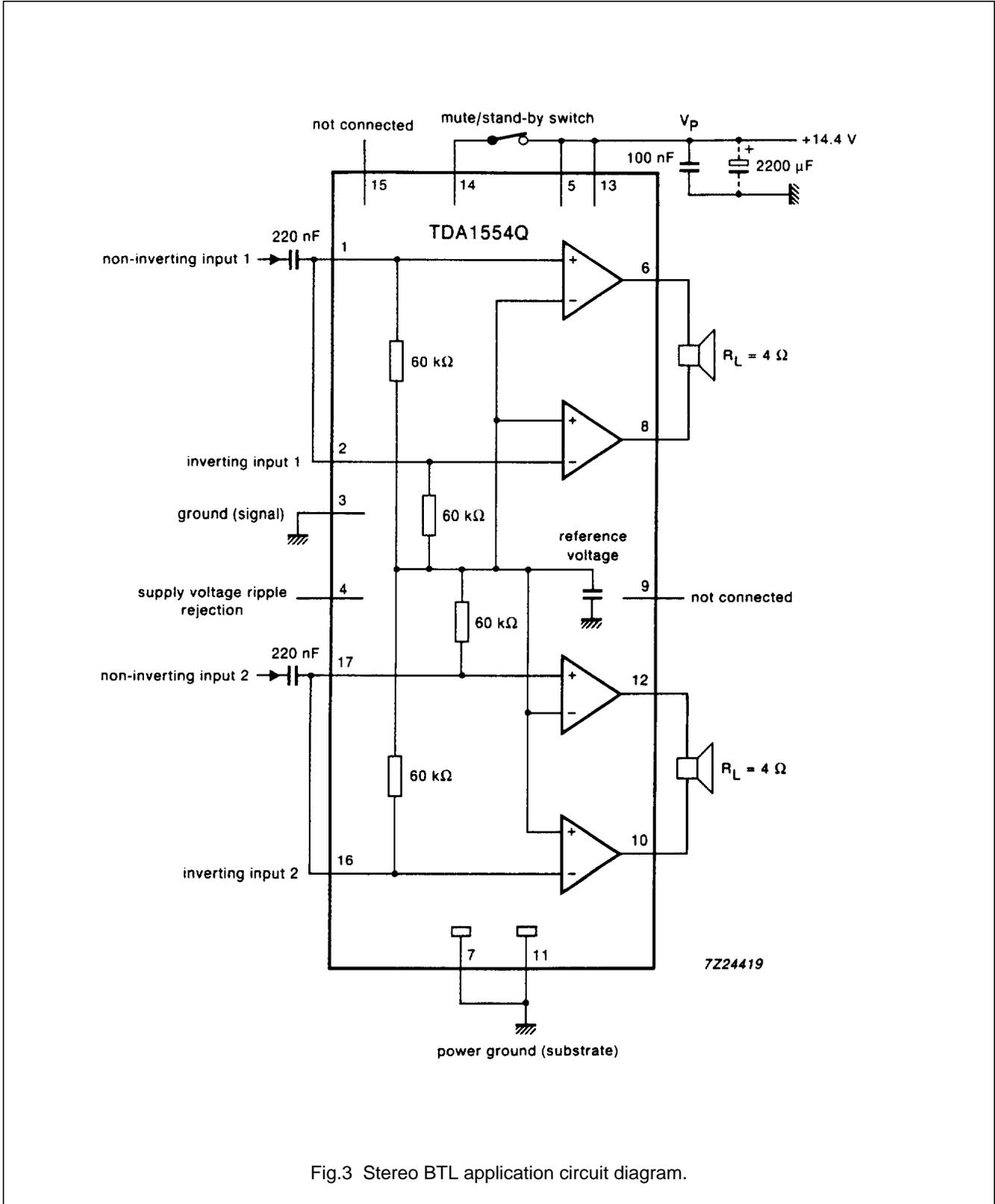
Fig.3 Stereo BTL application circuit diagram.
