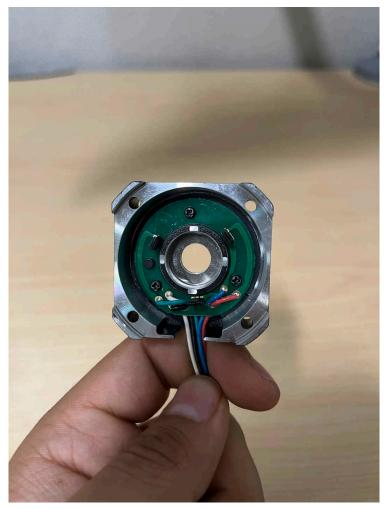
Figure 3-5. Hall Sensor Board Removal
