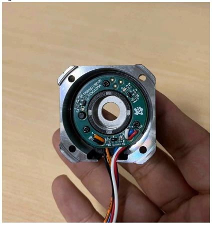
Figure 3-6. TMAG5115EVM on NEMA17 Motor Module
