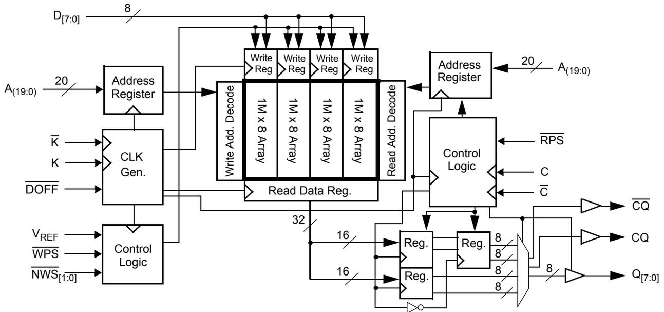
**Logic Block Diagram – CY7C1426KV18**
