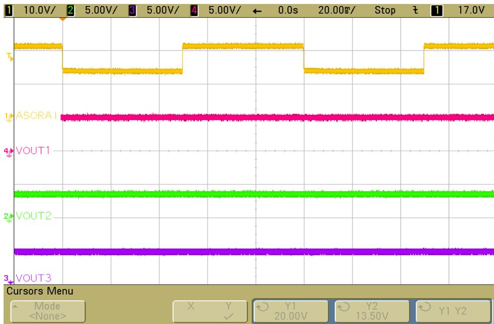
Figure 36. Output Response to OVS – VBAT-MON Left Open
