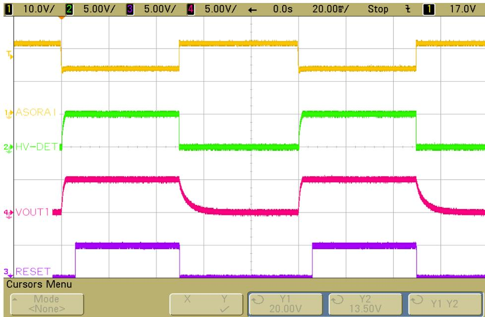
Figure 31. HV-DET Response to High Voltage – VBAT-MON tied to ASO-RAIL
