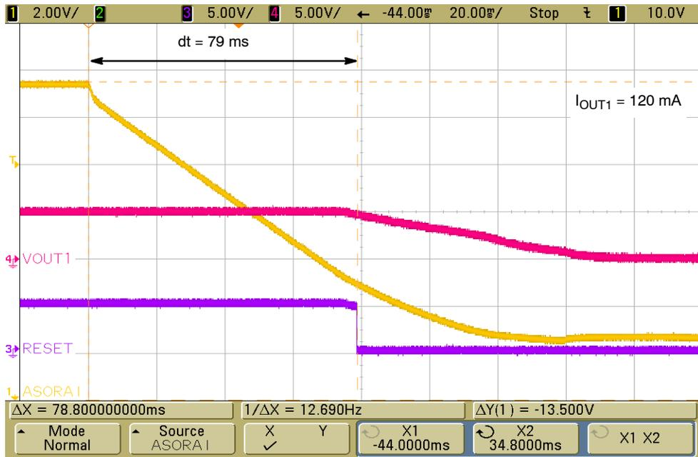
Figure 28. Output Response of LDO1 to Loss of Vin-B
