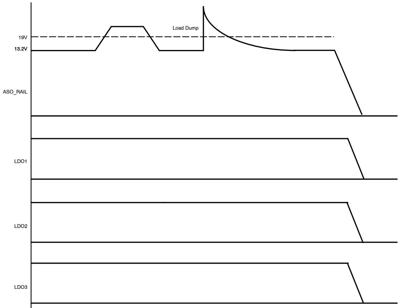
Figure 11. NCV8612B Regulator Output Timing Diagram- VBATT\_MON Grounded
