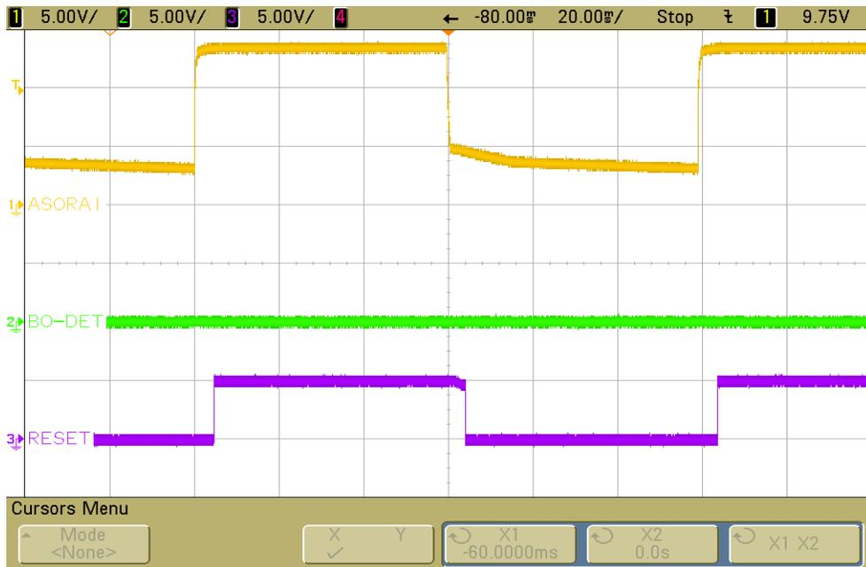
Figure 34. BO-DET Response to LOW Voltage – VBAT-MON Left Open
