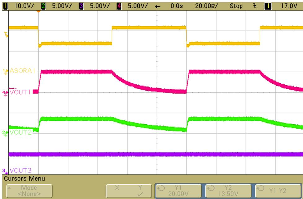
Figure 35. Output Response to OVS – VBAT-MON tied to ASO-RAIL
