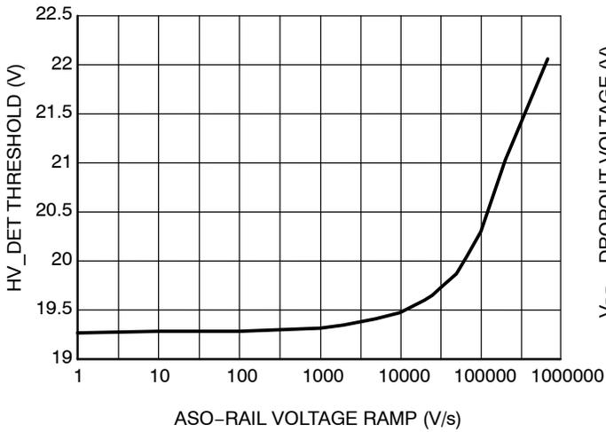
Figure 18. HV-DET Threshold vs. dV/dt
