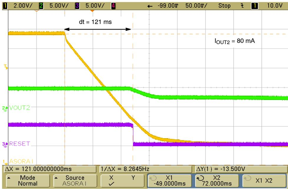
Figure 30. Output Response of LDO2 to Loss of Vin-B
