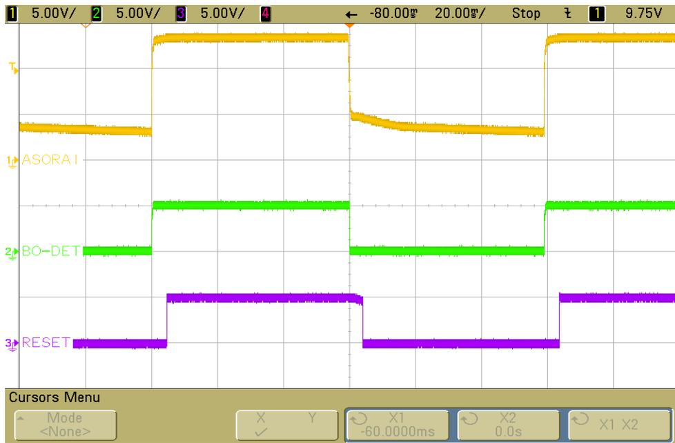
Figure 33. BO-DET Response to LOW Voltage – VBAT-MON tied to ASO-RAIL
