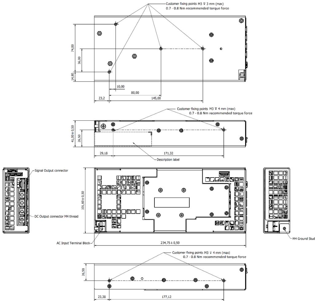
Figure 5. Mechanical Drawing - ACC750-1T24-PC / ACC750-1T48-PC Models
