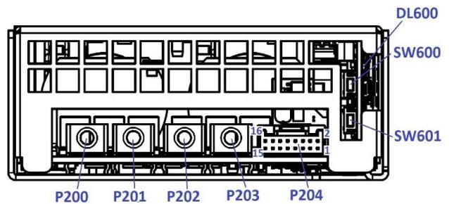
Figure 7. Rear View - ACC750-1T24-PC / ACC750-1T48-PC Models
