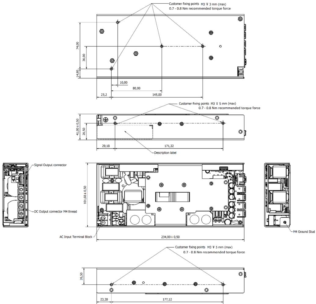
Figure 2. Mechanical Drawing – ACC750-1T24 / ACC750-1T48 Models
