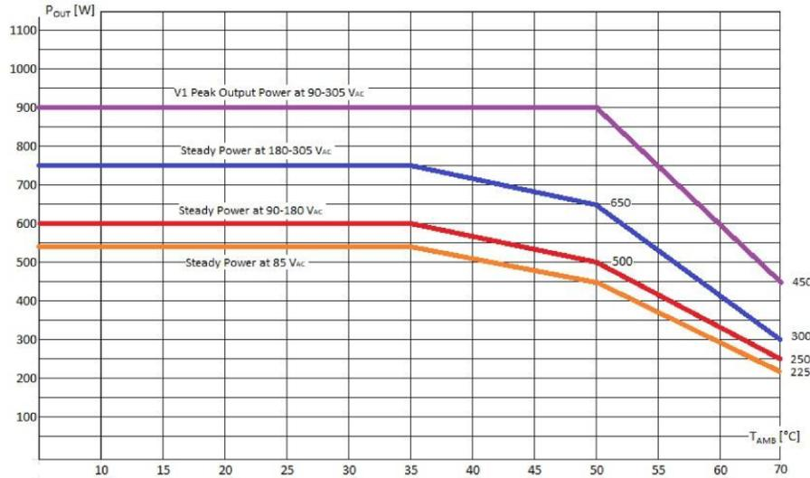
Figure 1 Derating Curves of ACC750 Series V1 P<sub>OUT</sub> to T<sub>AMB</sub>
