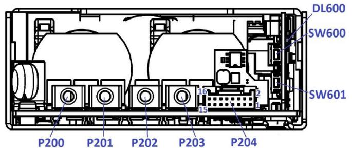
Figure 4. Rear View - ACC750-1T24 / ACC750-1T48 Models
