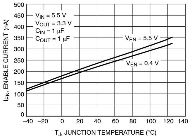
Figure 14. Current to Enable Pin vs. Temperature
