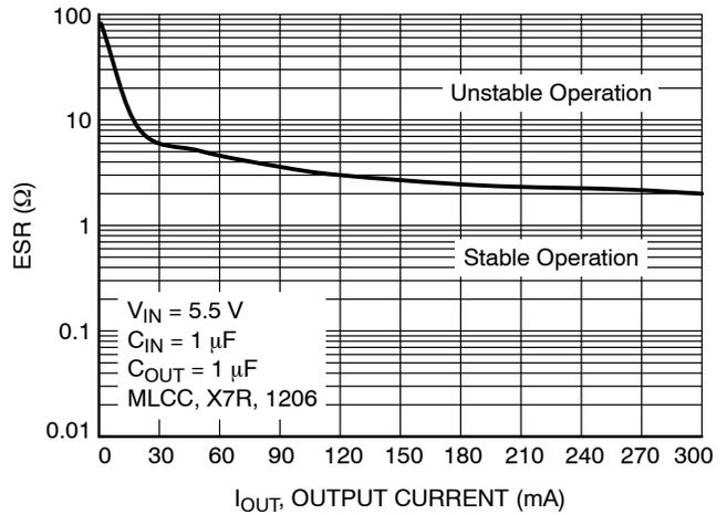
Figure 18. Output Capacitor ESR vs. Output Current
