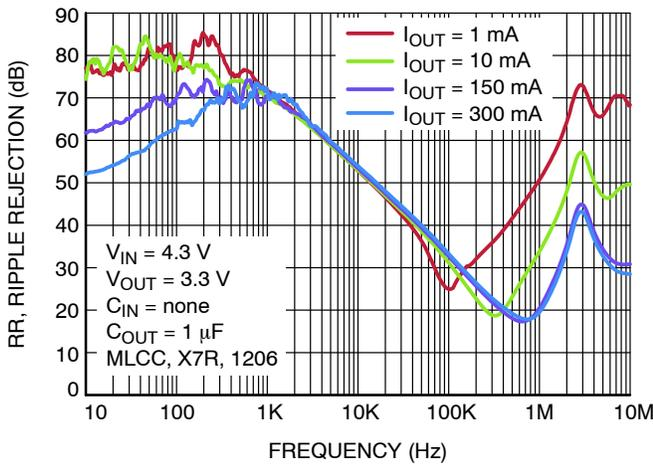
Figure 17. Power Supply Rejection Ratio - COUT = 1 μF
