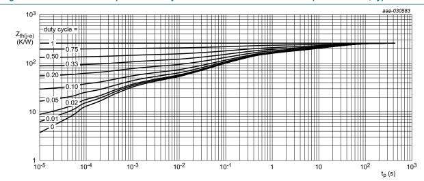
FR4 PCB; single-sided; 70 µm copper; tin-plated and standard footprint.
