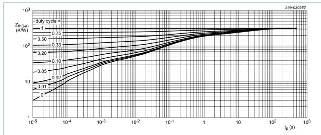
FR4 PCB; single-sided; 35 µm copper; tin-plated and standard footprint.
