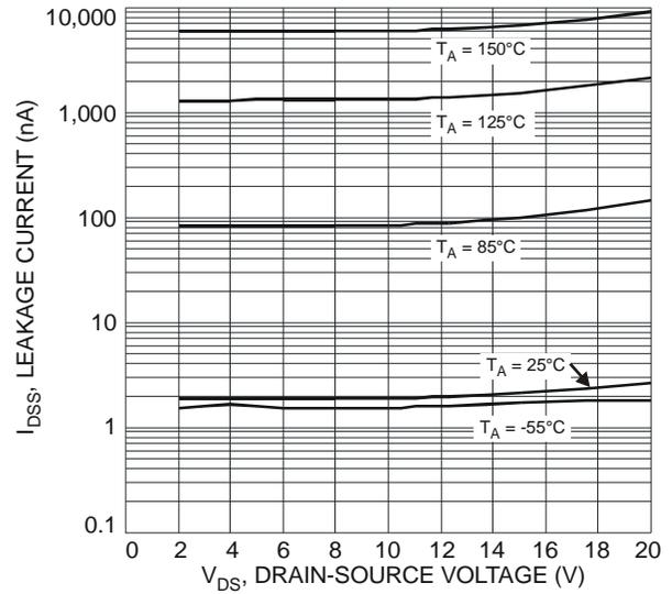
Fig. 10 Typical Drain-Source Leakage Current vs. Drain-Source Voltage
