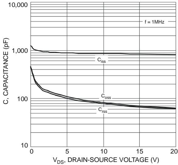
Fig. 9 Typical Capacitance
