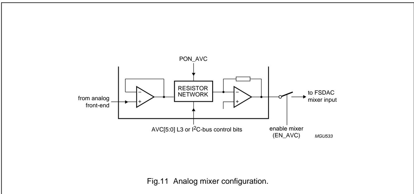
Fig.11 Analog mixer configuration.
