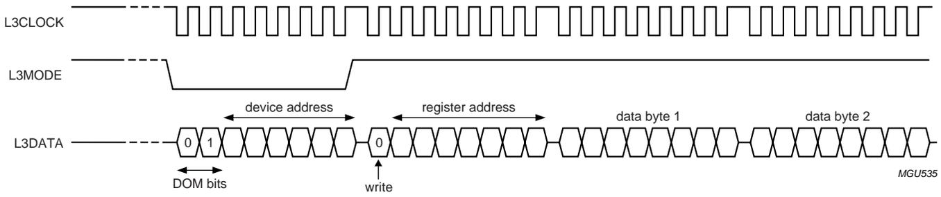
Fig.14 Data write mode for L3 version 2.
