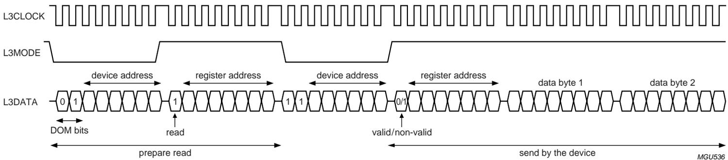
Fig.15 Data read mode for L3 version 2.
