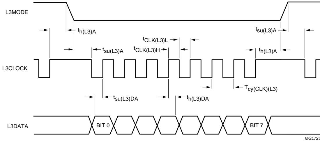
Fig.18 Timing of address mode.
