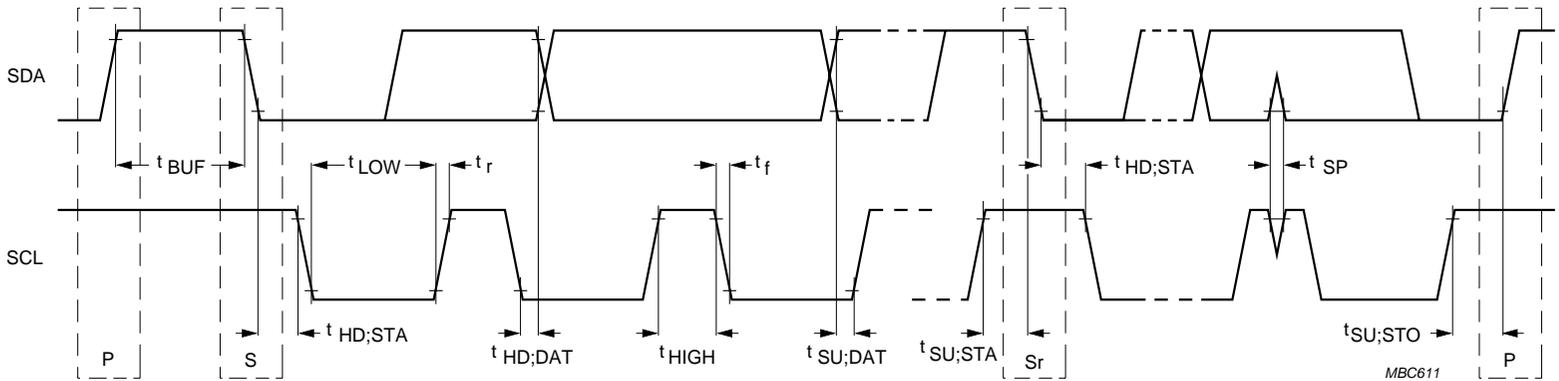
Fig.20 Timing of the I<sup>2</sup>C-bus transfer.
