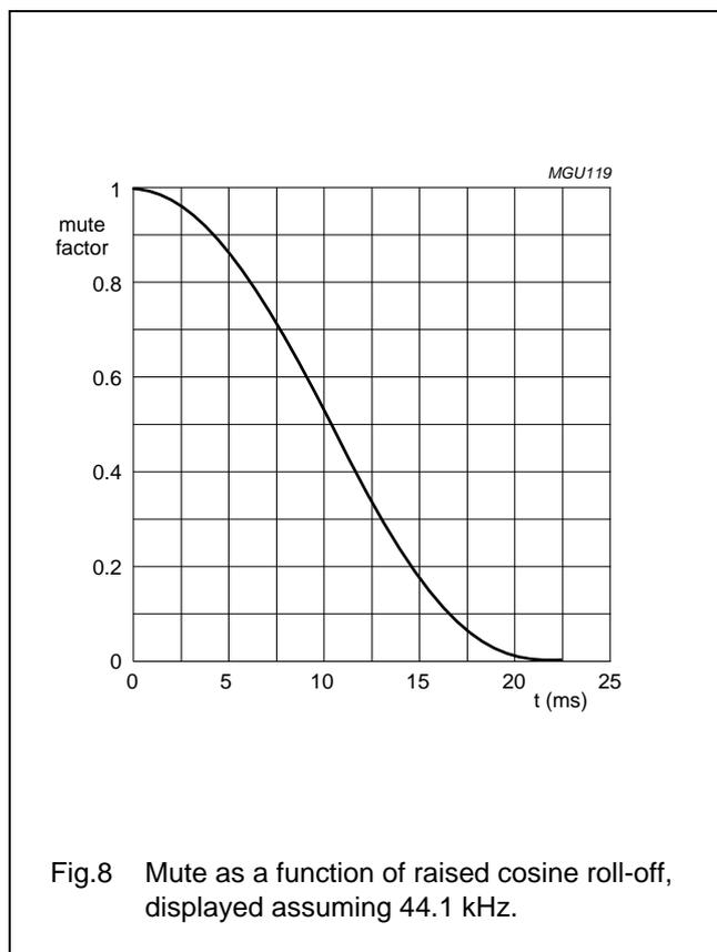
**Fig.8** Mute as a function of raised cosine roll-off, displayed assuming 44.1 kHz.
