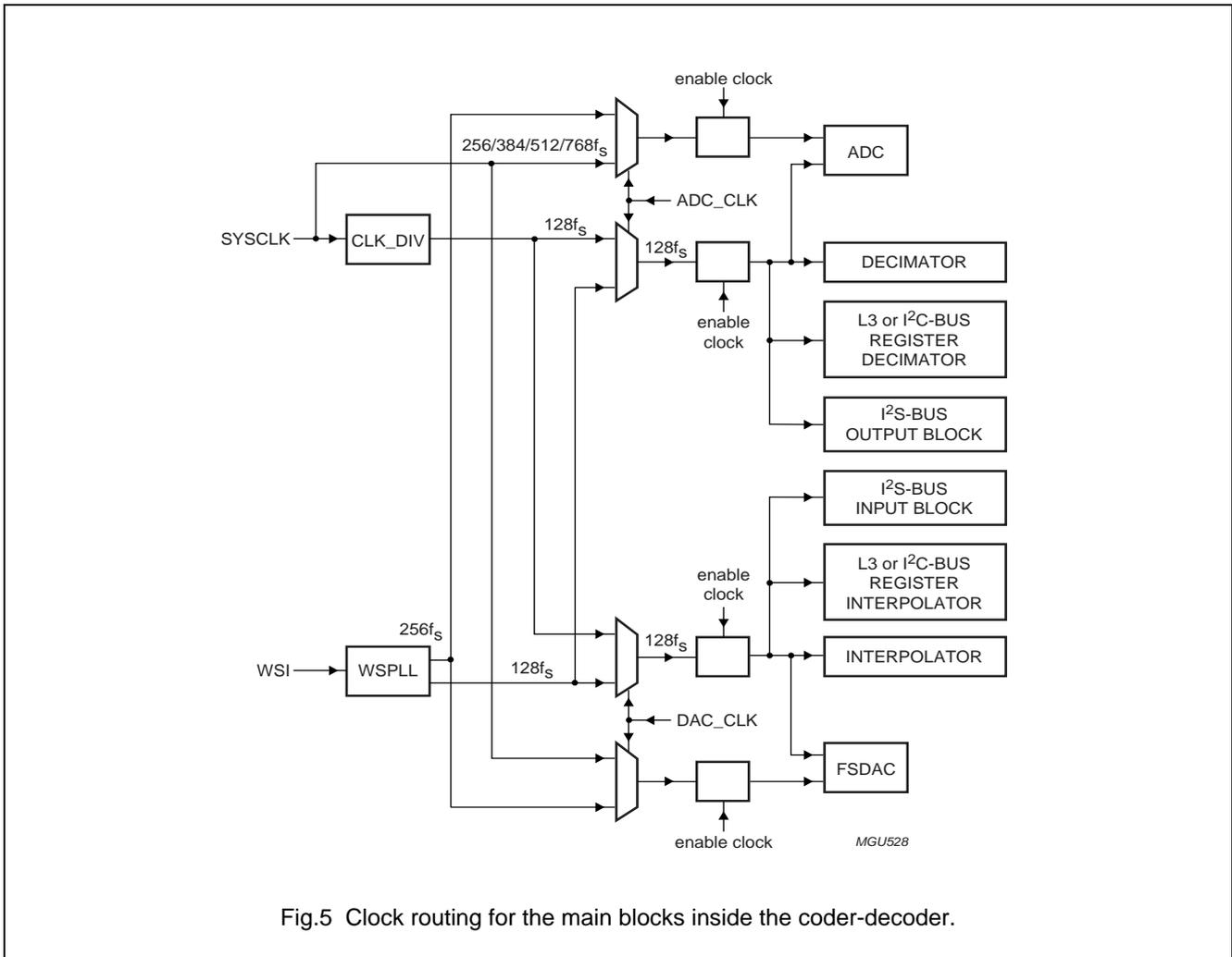
Fig.5 Clock routing for the main blocks inside the coder-decoder.
