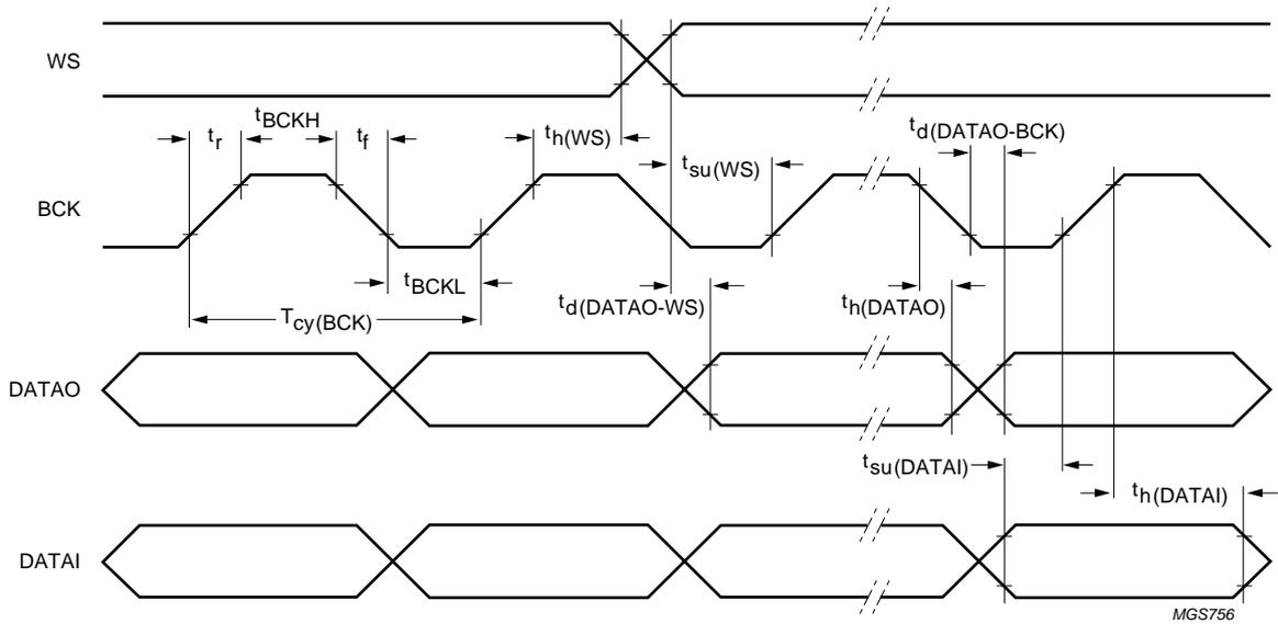
Fig.17 Serial interface input data timing.
