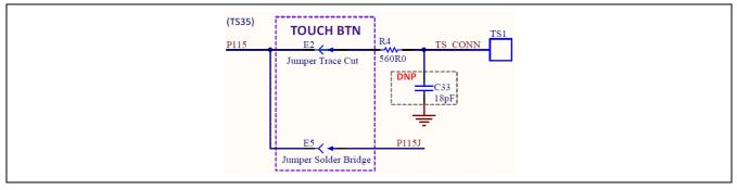
Figure 17 Capacitive touch button circuit
