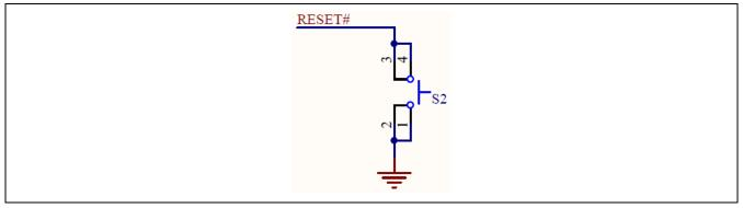
Figure 15 Reset switch circuit
