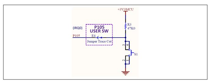
Figure 13 User switch circuit
