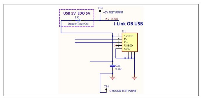
Figure 6 5 V power input circuit
