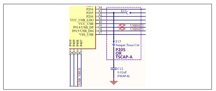
Figure 18 Capacitive touch TSCAP circuit
