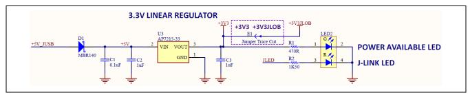
Figure 7 3.3 V power regulator circuit
