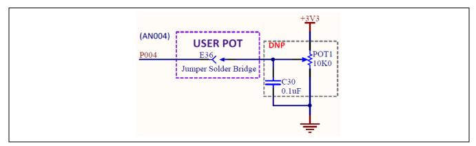
Figure 23 User potentiometer circuit
