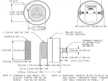
NOTE A: TERMINALS-.032 BRASS TIN PLATED, TAPPED FOR #6-32 SCREW. TWD #6-32 NICKEL PLATED BRASS SCREWS INCLUBED, WILL ACCEPT 1/4\* QUICK CONNECT. NOTE B: MOUNTING- REMOVE BLACK PLASTIC NUT AND INSERT THREADED FRONT THROUGH 1.25' HOLE PUNCHED IN PANEL, IF DRIENTATION IS NEEDED, NOTE LOCKING FLATS ON DRAWING. SCREW NUT BACK ON. DO NOT OVERTIGHTEN.
