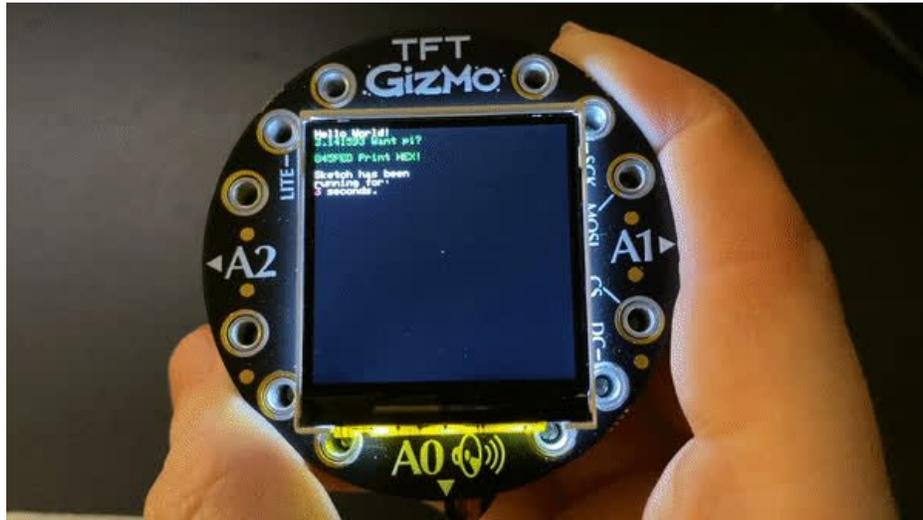
Once you've assembled the TFT Gizmo onto your Circuit Playground you can test it by loading one of these pre-made UF2 onto your Circuit Playground with the TFT Gizmo attached - it will perform a graphics test so you know that the Gizmo's attached!
