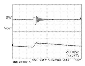
Fig.15 SW waveform Io=10mA
