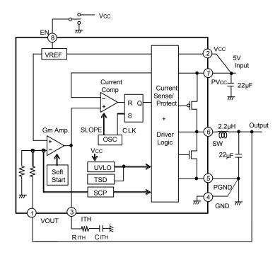
Fig.3 Block Diagram
