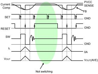
Fig.20 PWM switching timing chart
