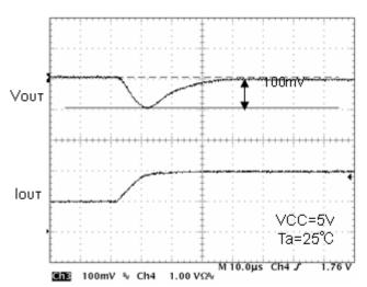
Fig.17 Transient response Io=1A→2A (10µs)
