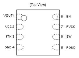
Fig.2 Pin Configuration
