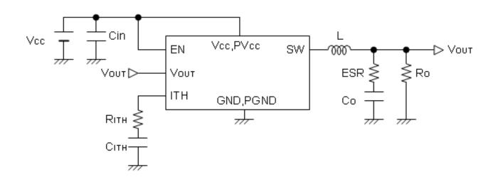
Fig.1 Typical Application Circuit
