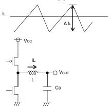
Fig.28 Output ripple current
