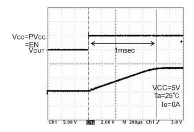
Fig.14 Soft start waveform
