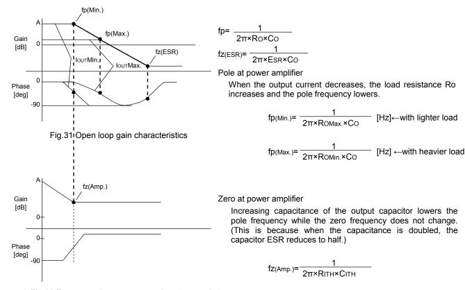
Fig.32 Error amp phase compensation characteristics
