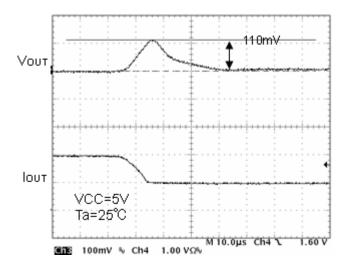
Fig.18 Transient response Io=2A→1A (10µs)
