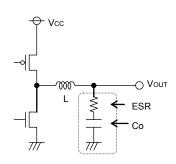
Fig.29 Output capacitor
