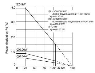
Ambient temperature:Ta [°C] Fig.27 Thermal derating curve (SON008V5060)
