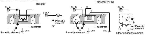
Fig.36 Simplified structure of monorisic IC
