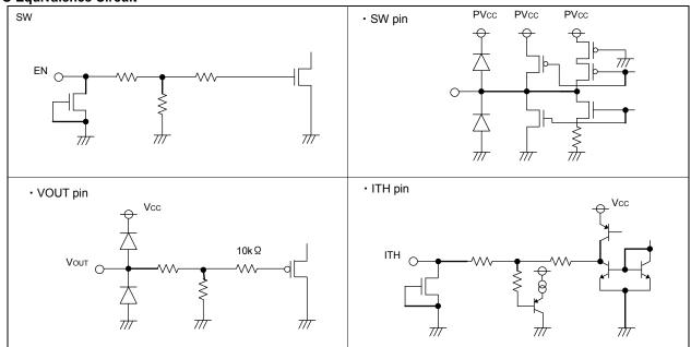
Fig.35 I/O equivalence circuit
