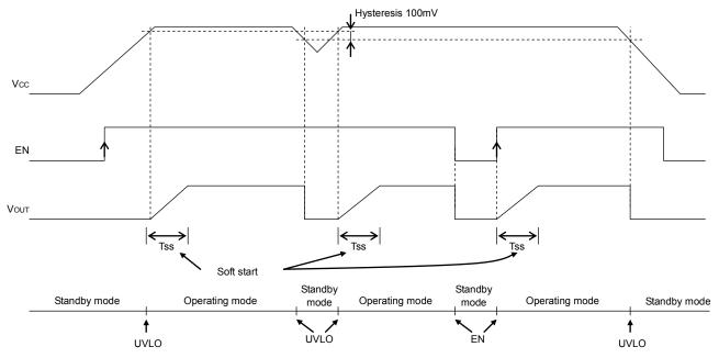
Fig.22 Soft start, Shutdown, UVLO timing chart
