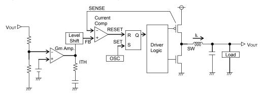
Fig.19 Diagram of current mode PWM control
