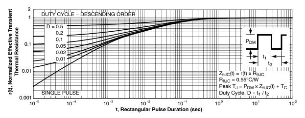
Figure 12. Transient Thermal Response Curve
