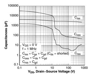
Figure 5. Capacitance Characteristics
