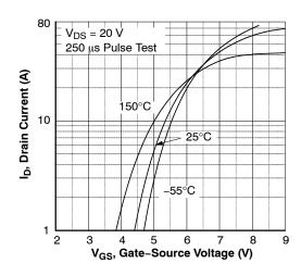
Figure 2. Transfer Characteristics
