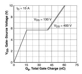
Figure 6. Gate Charge Characteristics
