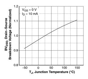
Figure 7. Breakdown Voltage Variation vs. Temperature
