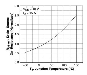
Figure 8. On–Resistance Variation vs. Temperature
